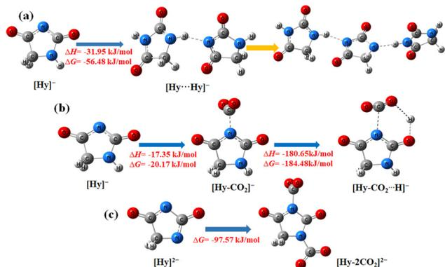
Fig. 1 The optimized geometry and the calculated energy. (a) Chain-like intermolecular hydrogen bonding of  $[\text{Hy}]^-$ ; (b)  $\text{CO}_2$  absorption by  $[\text{Hy}]^-$  and quasi-intramolecular cyclic hydrogen bonds formed by  $[\text{Hy}-\text{CO}_2]^-$  and the active hydrogen atom; (c) double-site interaction between  $[\text{Hy}]^-$  and  $\text{CO}_2$ .
