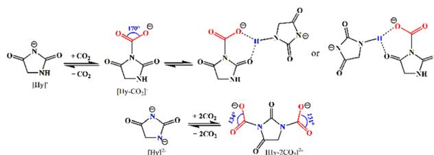
Scheme 2 Possible mechanism of  $\text{CO}_2$  absorption by  $[\text{P}_{4442}][\text{Hy}]$  and  $[\text{P}_{4442}]_2[\text{Hy}]$ .
