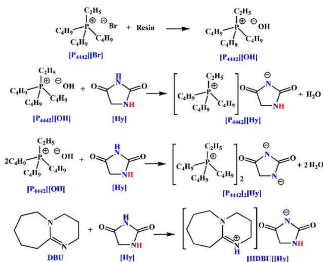
Scheme 1 Synthesis of [P<sub>4442</sub>][Hy], [P<sub>4442</sub>]<sub>2</sub>[Hy], and [HDBU][Hy].
