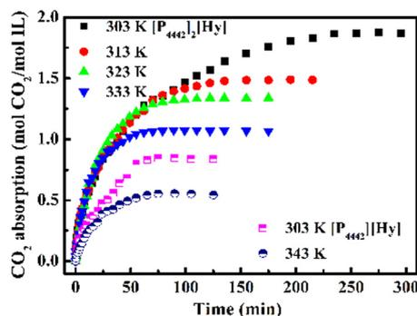
Fig. 3  $\text{CO}_2$  absorption behavior of  $[\text{P}_{4442}][\text{Hy}]$  and  $[\text{P}_{4442}]_2[\text{Hy}]$  at 0.1 MPa.
