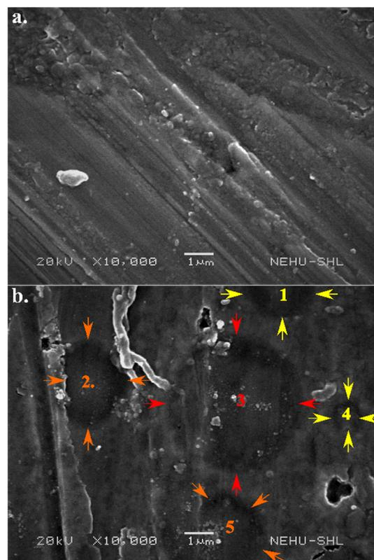
Fig. 5 SEM images showing the surface of electrodes post-ablation at (a)  $0 \text{ V m}^{-1}$  and (b)  $3750 \text{ V m}^{-1}$  deposition. To divulge more, the Cu electrode where  $\text{Mn}_2\text{O}_3$  gets deposited ( $0^\circ$ – $45^\circ$ ) is characterized using SEM.
