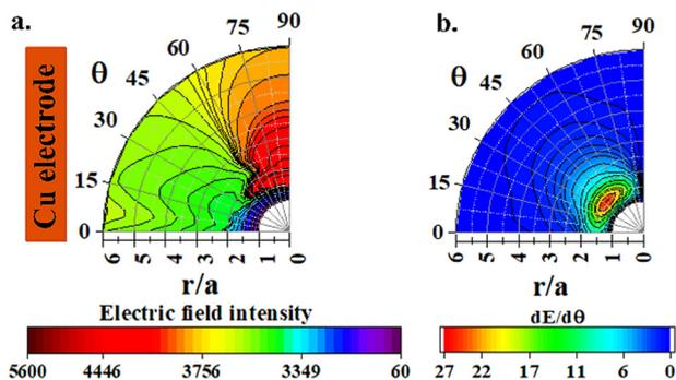
Fig. 8 (a) Electric field intensity outside the macro bubble at  $3750 \text{ V m}^{-1}$ . (b) An angular gradient of electric field intensity at  $3750 \text{ V m}^{-1}$ .
