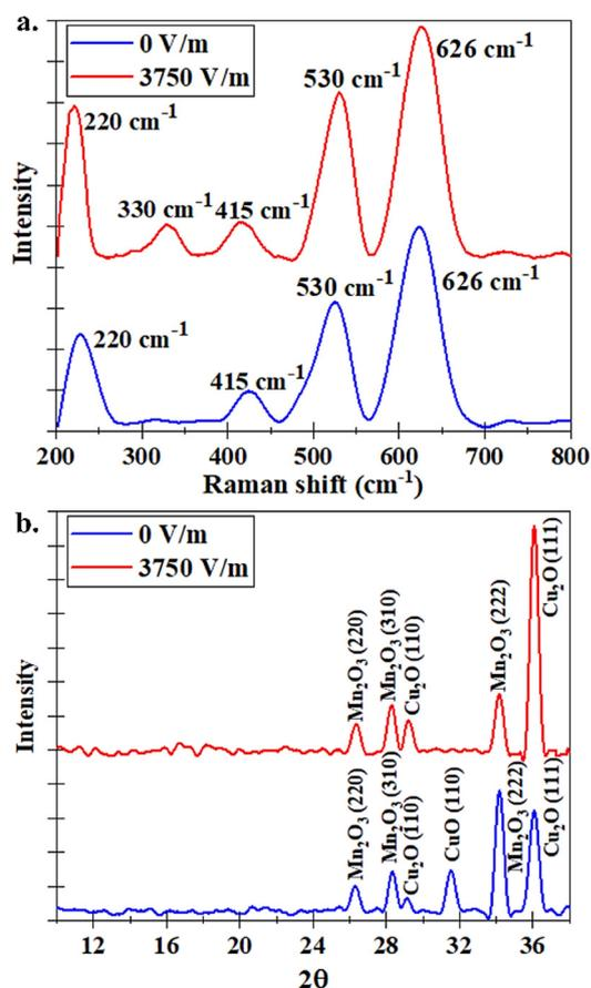
Fig. 4 (a) Micro-Raman spectra of the electrodes without ( $0 \text{ V m}^{-1}$ ) and with ( $3750 \text{ V m}^{-1}$ ) applied electric field. (b) XRD pattern of the electrodes at an applied electric field of  $0 \text{ V m}^{-1}$  and  $3750 \text{ V m}^{-1}$ .
