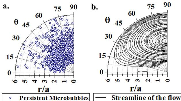
Fig. 7 (a) Coordinates of the microbubble at  $0 \text{ V m}^{-1}$ . (b) Simulated streamline flow of the microbubbles induced by the oscillations of the macro bubble at  $0 \text{ V m}^{-1}$ .
