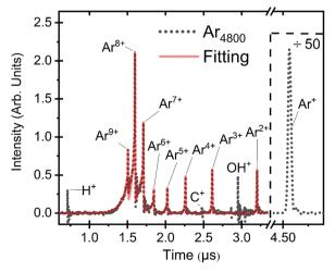
Fig. 3 Time-of-flight spectrum of neat clusters of  $Ar_{4800}$ . The TOF profiles of each MCAI with +2 to +9 charges are fitted using eqn (1) (see text for details), and the composite from individual ions is shown as the red continuous line. Ions with charges above +9 are ignored.
