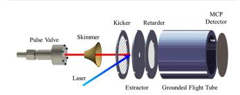
Fig. 1 Experimental setup showing the electrodes for the time-of-flight mass spectrometer. The Retarder electrode is only added for the experiment of investigating the effect of the electric field between the Kicker and
