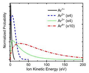
Fig. 4 Kinetic energy distributions of Ar ions with +1 to +4 charges from neat clusters of Ar<sub>4800</sub>. The distributions of MCAI are scaled up to show their detailed features
