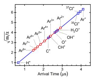
Fig. 2 Mass-time correlation of ions observed from the background and from clusters  $Ar_{800}3ClB_{0.07}$ . The blue continuous line is the fitting result from the singly charged atomic ions found in the background and the signal (blue squares), and the red circles are the corresponding arrival time of the multiply charged atomic ions from the clusters.
