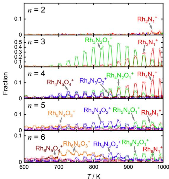
Fig. 4 Intensity changes of one-O-atom-deficient  $\text{Rh}_n\text{N}_x\text{O}_{x-1}^+$  ( $n = 2-6$ ), the main products of the reduction reaction by CO, as a function of temperature in the range of 600–1000 K. Intensities in the presence and absence of CO are depicted by open and filled circles, respectively. The number of N atoms in the cluster is color-coded as red, green, blue, orange, brown, purple, and pink.
