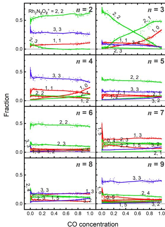
Fig. 5 Fractions of  $\text{Rh}_n\text{N}_x\text{O}_y^+$  clusters ( $n = 2-9$ ) produced by the reaction of CO at 903 K as a function of CO concentration. Lines in the plots were added for visibility. The colors khaki, red, green, and blue correspond to compositions containing zero, one, two, and three N atoms, respectively.
