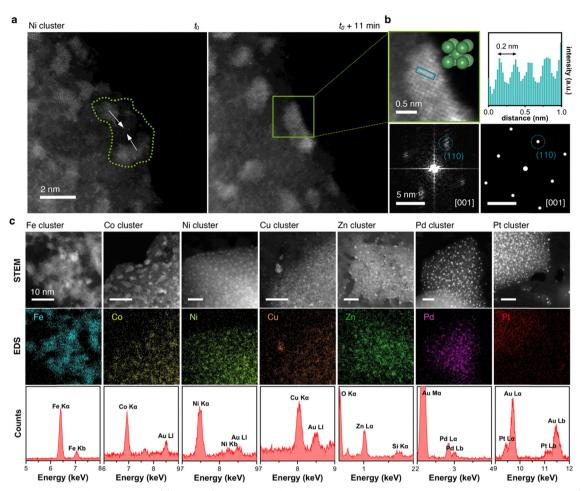
Fig. 7 STEM mode analysis of metal clusters. (a) HAADF-STEM images of the coalescing crystalline Ni clusters upon irradiating the area in STEM mode for 11 min. (b) Magnified HAADF-STEM image of the BCC Ni crystal, the measured plot profile and experimental FFT (left) and simulated (right) diffraction pattern. (c) HAADF-STEM images and EDS mapping of all investigated metals (Fe, Co, Ni, Cu, Zn, Pd, Pt) and clusters.
