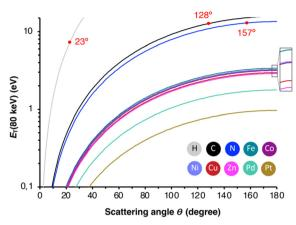
Fig. 4 Transferred energy  $E_T$  against the elastic scattering angle  $\Theta$  for all studied elements. In red are the angles indicated, at which  $E_T$  exceeds  $E_d$ .
