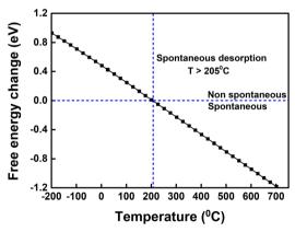
Fig. 4 The free energy change for the desorption of an HCl molecule from the NH<sub>3</sub><sup>+</sup>Cl<sup>-</sup> surface site in **P1b** as a function of temperature.
