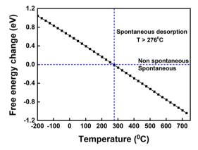
Fig. 7 The free energy change for the desorption of an HCl molecule from the NH<sub>3</sub>+Cl<sup>-</sup> surface site in **P2** as a function of the temperature.
