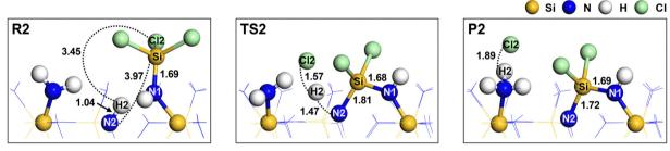
Fig. 6 The atomistic structures for the reactant (R2), transition (TS2), and product (P2) states of the second Si-N bond formation reaction. The dotted lines represent the interatomic distances with corresponding values displayed in Å. The bond lengths are also shown in Å.
