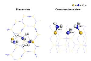
Fig. 1 The atomistic structure of the  $-NH_2^*$  and  $-NH^*$  terminated silicon nitride surface with the reaction sites. In the planar view, the dotted lines represent the interatomic distances with corresponding values in Å. In the cross-sectional view, the N-H bond lengths are shown in Å.
