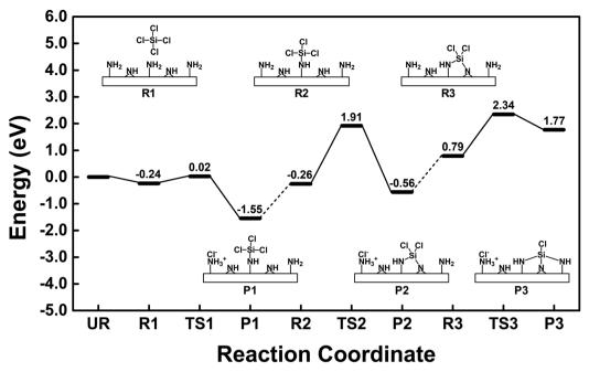
Fig. 5 Energy diagram for the chemisorption of SiCl<sub>4</sub> on silicon nitride
