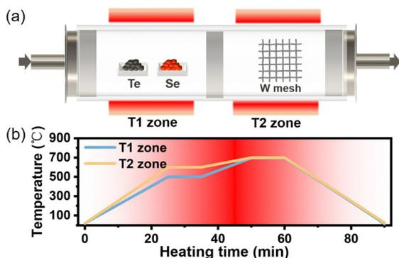
Fig. 1 (a) Schematic illustration of the high-temperature reaction system used for the synthesis of Te- $\text{WSe}_2$ . (b) Temperature–time profiles for the synthesis of Te- $\text{WSe}_2$ .
