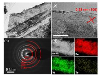
Fig. 3 (a) and (b) HRTEM images of Te-WSe<sub>2</sub>. (c) SAED pattern of Te-WSe2. (d) STEM-HAADF with EDS elemental mapping images of Se, W, Te.
