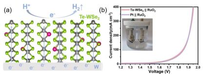
Fig. 7 (a) Schematic diagram showing electron transport in Te-WSe<sub>2</sub>/W. (b) Polarization curves of two-electrode overall water splitting performed in 0.5 M H<sub>2</sub>SO<sub>4</sub> at a scanning rate of 5 mV s<sup>-1</sup>. RuO<sub>2</sub> serves as the anode, while Te-WSe<sub>2</sub> and Pt/C are employed as cathodes, respectively. Inset: A photograph of the overall water splitting system
