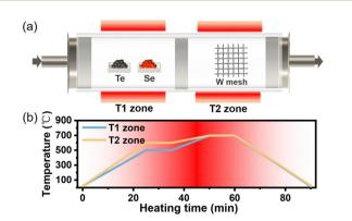
Fig. 1 (a) Schematic illustration of the high-temperature reaction system used for the synthesis of Te-WSe<sub>2</sub>. (b) Temperature-time profiles for the synthesis of Te-WSe<sub>2</sub>
