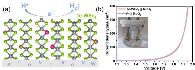
Fig. 7 (a) Schematic diagram showing electron transport in Te-WSe<sub>2</sub>/W. (b) Polarization curves of two-electrode overall water splitting performed in 0.5 M H<sub>2</sub>SO<sub>4</sub> at a scanning rate of 5 mV s<sup>-1</sup>. RuO<sub>2</sub> serves as the anode, while Te-WSe<sub>2</sub> and Pt/C are employed as cathodes, respectively. Inset: A photograph of the overall water splitting system.
