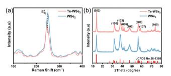
Fig. 5 (a) and (b) Raman scattering spectra and XRD pattern of Te-WSe<sub>2</sub> and WSe2. The curves denoted with pink and blue colors correspond to signals from Te-WSe2 and WSe2.
