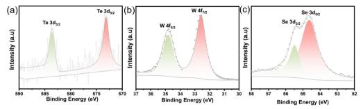
Fig. 4 XPS spectra of Te-WSe<sub>2</sub> showing the signals of (a) Te 3d, (b) W 4f and (c) Se 3d
