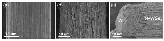
Fig. 2 (a) SEM image of the original W mesh. (b) and (c) SEM images of Te-WSe<sub>2</sub>/W.
