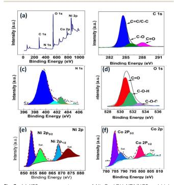
Fig. 3 (a) XPS survey spectrogram of Ni-Co-LDH NTA/NGS and highresolution deconvoluted XPS spectra of (b) C 1s, (c) N 1s, (d) O 1s, (e) Ni 2p and (f) Co 2p of Ni-Co-LDH NTA/NGS
