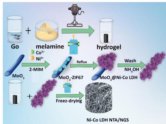
Scheme 1 Illustration of the Ni-Co-LDH NTA/NGS preparation process.
