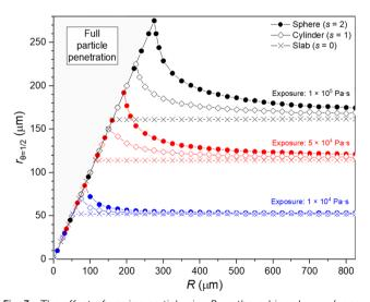
Fig. 3 The effect of varying particle size R on the achieved  $r_{\theta=1/2}$  (penetration depth) with three different exposures of reactant (1  $\times$  10<sup>4</sup>, 5  $\times$  10<sup>4</sup> and  $1 \times 10^5$  Pa s). Three curves for each exposure present the model results for different shape factors: sphere (s = 2), cylinder (s = 1) and slab (s = 0). The simulation parameters are presented in Tables 1 and 2.
