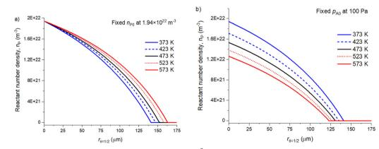
Fig. 8 The effect of selecting the volumetric reactant number density (m<sup>-3</sup>) or partial pressure (Pa) in a diffusion-reaction model as a function of temperature. Panel (a) shows the fixed volumetric reactant number density to  $1.94 \times 10^{22} \, \mathrm{m}^{-3}$  and (b) shows the fixed partial pressure to 100 Pa as a function of the achieved penetration depth  $(r_{\theta=1/2})$ . A full list of the simulation parameters and plotted values are presented in the ESI† in Table S4.
