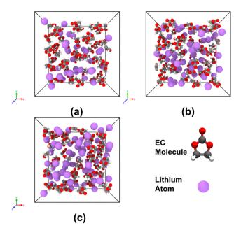
Fig. 1 Illustration of simulation system configurations: (a) system 1 with 60 EC and 40 Li atoms. (b) System 2 with 60 EC and 60 Li atoms. (c) System 3 with 60 EC and 80 Li atoms. Colour code: C: grey, H: white, O: red, Li: purple.
