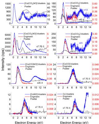
Fig. 1 The DEA products of Co(CO)<sub>3</sub>NO obtained from CLUSTER-ILN measurements (blue lines) compared with previously published experiments: gas-phase date<sup>17,19</sup> (red lines), He clusters data<sup>21</sup> (grey circles). The y-axis on the left represents the intensities of CLUSTER-ILN data, while the intensities from previous works<sup>17,19</sup> (with scaling factors) are on the right.
