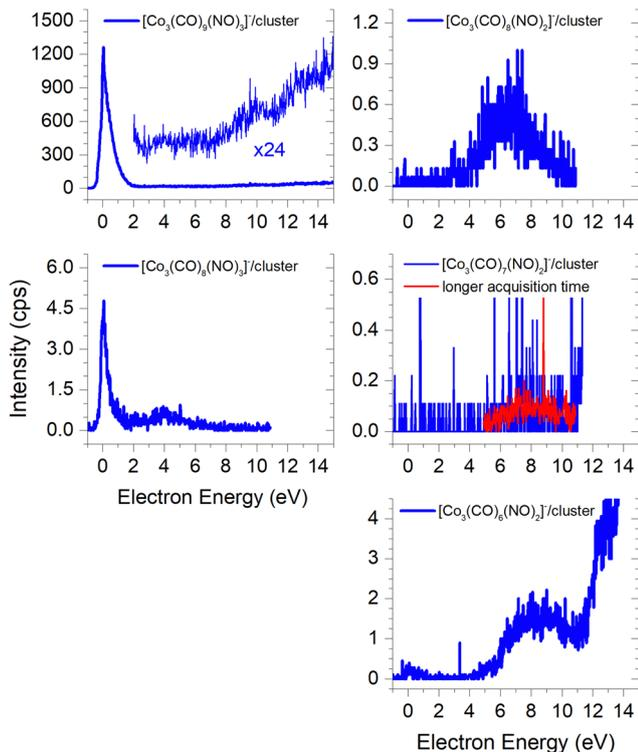
Fig. 3 The molecular trimer  $[M_3]^-$  and the associated clusters of two molecules ( $M_2$ ) with the DEA products  $[\text{Co}(\text{CO})_2\text{NO}]^-$ ,  $[\text{Co}(\text{CO})_2]^-$ ,  $[\text{CoCO}]^-$  and  $\text{Co}^-$ .
