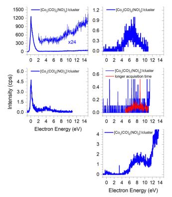
Fig. 3 The molecular trimer  $[M_3]^-$  and the associated clusters of two molecules (M<sub>2</sub>) with the DEA products [Co(CO)<sub>2</sub>NO]<sup>-</sup>, [Co(CO)<sub>2</sub>]<sup>-</sup>, [CoCO] and Co
