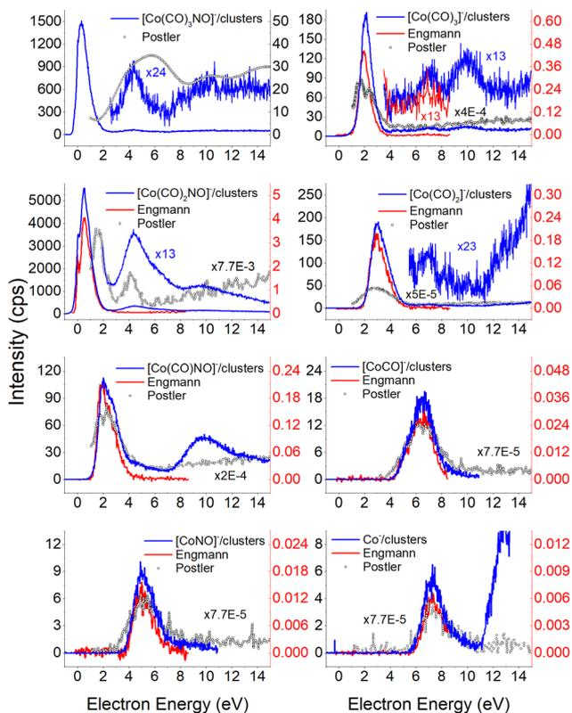
Fig. 1 The DEA products of  $\text{Co}(\text{CO})_3\text{NO}$  obtained from CLUSTER-ILN measurements (blue lines) compared with previously published experiments: gas-phase data<sup>17,19</sup> (red lines), He clusters data<sup>21</sup> (grey circles). The y-axis on the left represents the intensities of CLUSTER-ILN data, while the intensities from previous works<sup>17,19</sup> (with scaling factors) are on the right.
