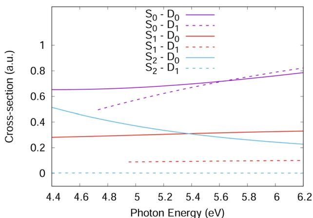
Fig. 4 One-photon photo-ionisation cross-sections of phenol as a function of incident photon energy corresponding to ionisation from  $S_1$  and  $S_2$  to  $D_0$  and  $D_1$ . For ionisation from  $S_0$ , the cross-section for the two-photon process is shown.
