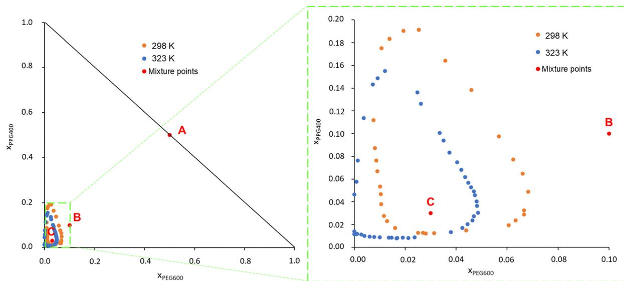
Fig. 1 Experimental phase diagrams for the system PEG600/PPG400/H<sub>2</sub>O at 298 K and 323 K, and atmospheric pressure.  $X_{\text{PEG600}}$  and  $X_{\text{PPG400}}$  are the mole fractions of PEG600 and PPG400, respectively. The mixture points A, B and C correspond to the MD compositions further studied and analyzed along this work.
