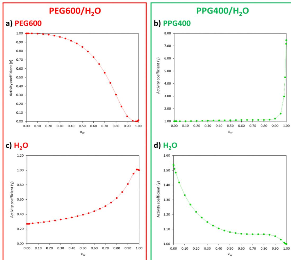
Fig. 7 Activity coefficients ( $\gamma$ ) of PEG600 (a), PPG400 (b) and water (c) and (d) for different  $x_w$  of the PEG600/H<sub>2</sub>O and PPG400/H<sub>2</sub>O systems calculated with COSMO-RS at 298.15 K.
