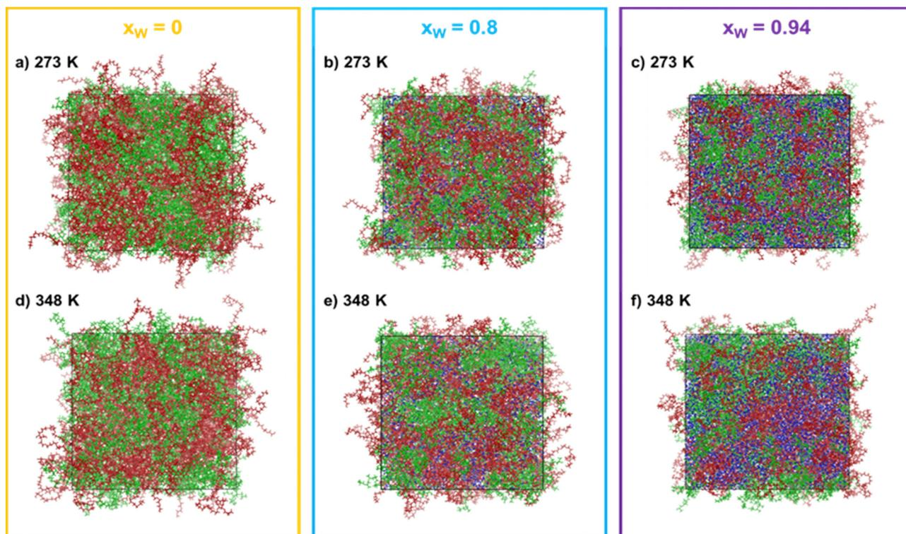
Fig. 2 Snapshots from MD simulations containing 1:1 molar ratio between PEG600 and PPG400 for increasing water concentrations [ $x_w = 0$  (yellow box),  $x_w = 0.8$  (blue box) and  $x_w = 0.94$  (purple box)], at 273 K ((a), (b) and (c)) and 348 K ((d), (e) and (f)). PEG600, PPG400 and water are represented by red, green and blue colors, respectively.
