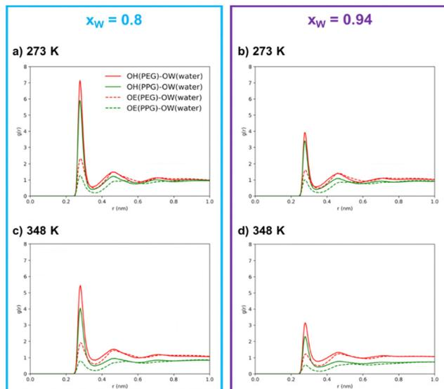
Fig. 4 Radial distribution functions between oxygen atoms belonging to PEG600/PPG400 and water for increasing water concentrations ( $x_w = 0.8$  (blue box) and  $x_w = 0.94$  (purple box)), at 273 K ((a) and (b)) and 348 K ((c) and (d)). "OE" represents ether group oxygen atoms and "OH" represents terminal hydroxyl groups while OW is the oxygen of water molecules.
