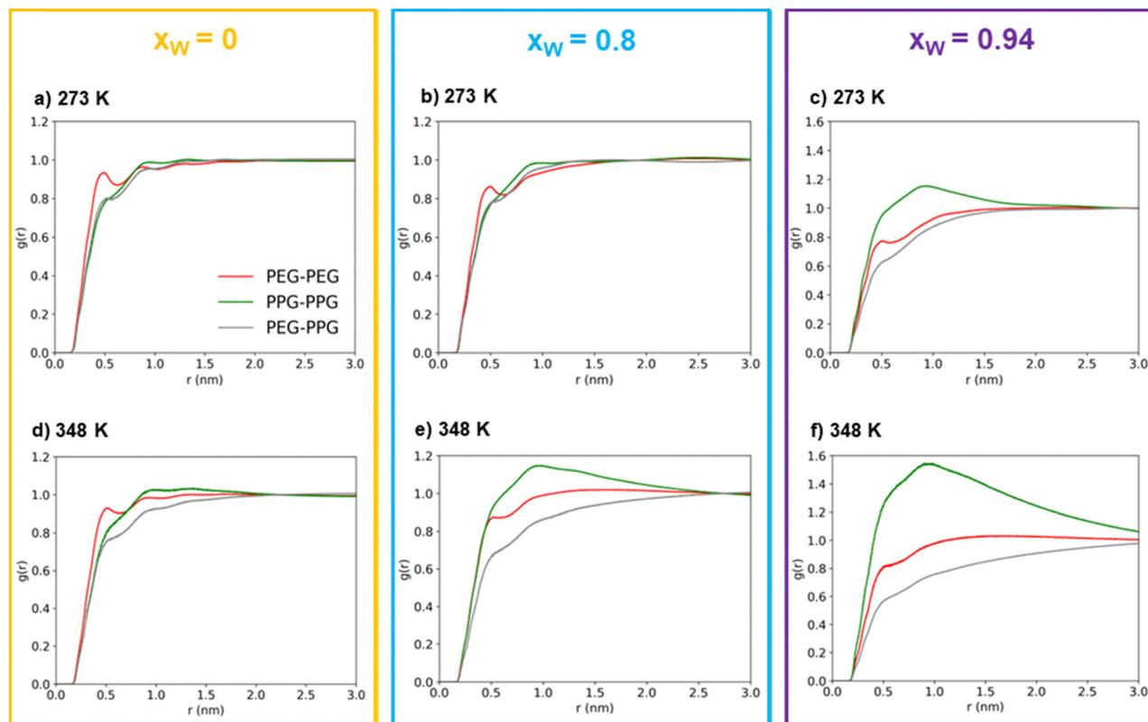
Fig. 3 Atom-wise polymer-polymer intermolecular radial distribution functions obtained from MD simulations for increasing water concentrations [ $x_w = 0$  (yellow box),  $x_w = 0.8$  (blue box) and  $x_w = 0.94$  (purple box)], at 273 K ((a), (b) and (c)) and 348 K ((d), (e) and (f)). The red, green and gray curves correspond to PEG600-PEG600, PPG400-PPG400 and PEG600-PPG400 pairs, respectively.
