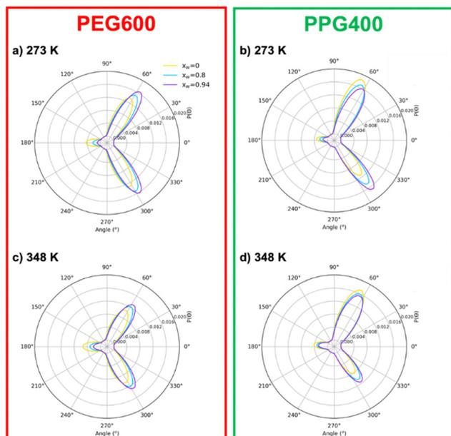
Fig. 5 Probability distribution for the O–C–C–O dihedral for PEG600 and PPG400 as a function of water content ( $x_W = 0$ , yellow line;  $x_W = 0.8$ ; blue line;  $x_W = 0.94$  purple line) at 273 K (a) and (b) and 298 K (c) and (d), obtained from the MD trajectories.
