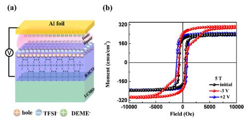
Fig. 4 (a) Schematic illustration of the device for ionic liquid gating. (b) Moment as a function of the magnetic field of the B-SCO/LCMO bilayer after being gated by different bias voltages.
