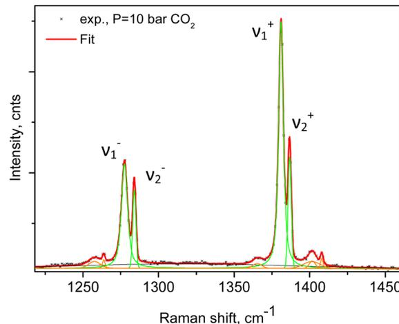
Fig. 3 Linear least-squares fitting of the experimental data at 10 bar CO<sub>2</sub> using a series of pseudo-Voigt profiles. Green-coloured lines depict the individual peak components and the red line is the total fit. The two pairs of "hot" lines due to scattering from molecules in excited states could be clearly seen and were also explicitly taken into account.
