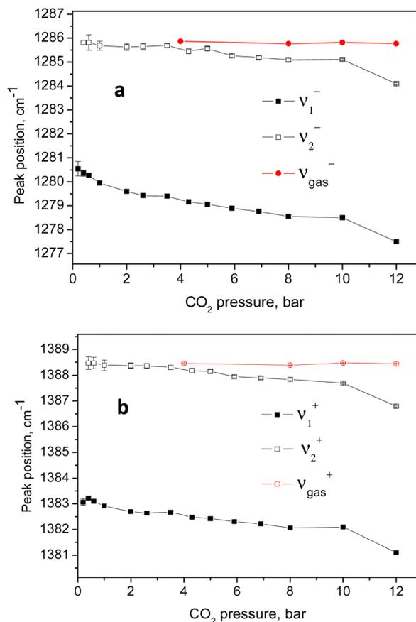
Fig. 6 Variation of the positions of the higher and lower energy parts of the two Fermi diads with the CO<sub>2</sub> equilibrium pressure.
