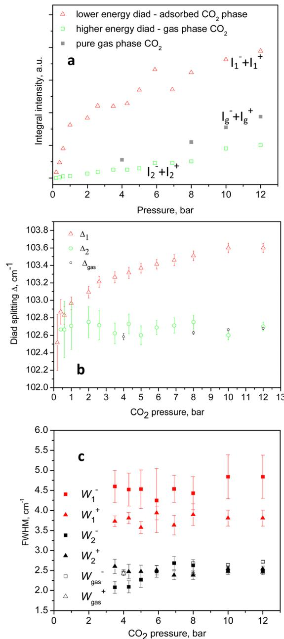
Fig. 5 Observed spectral lines integral intensities in the (a)-block, and the Fermi diads splitting in (b). The (c)-block shows the corresponding line widths denoted as *W*'s. All sets of data as functions of the loading CO<sub>2</sub> pressure, including those in the pure gas-phase data, as indicated in the figure legends.
