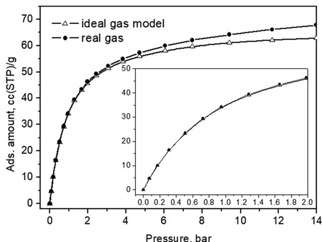
Fig. 8 CO<sub>2</sub> adsorption isotherm of the Silicalite-1 sample measured at 299 K. The same data, up to a pressure of 2 bar, are shown in the inset.
