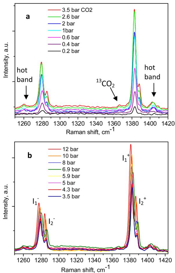
Fig. 2 Raman spectra of CO<sub>2</sub>-loaded Silicalite-1 taken at 299 K and variable pressures: (a) between 0.2 and 3.5 bar; (b) up to 12 bar, as indicated in the figure legends.
