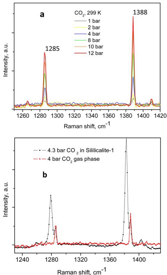
Fig. 4 Variable pressure gas-phase Raman spectra of CO<sub>2</sub> compressed within a total flight path of about 4 mm (forward + back) (a); spectra at about 4 bar equilibrium pressure in both the adsorbed and gas phases are shown together in (b).
