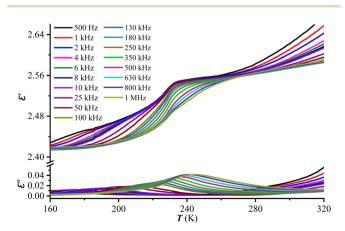
Fig. 4 Temperature-dependent  $\varepsilon'$  and  $\varepsilon''$  of **1** at various ac frequencies
