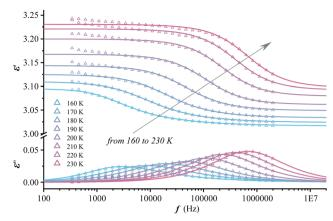
Fig. 5 Frequency-dependent  $\varepsilon'$  and  $\varepsilon''$  for **1** at several selected temperatures (a), and the Cole-Cole diagrams are plotted as a series of arcs to show the relationship between  $\varepsilon'$  and  $\varepsilon''$  (b). Solid curves represent the fit of the experimental data to the Debye equation.
