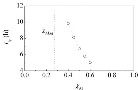
Fig. 6 The ignition time,  $t_{ig}$ , of Al–Ni powder mixtures as a function of the Al atomic fraction,  $\chi_{Al}$ . The best-fitted curve and the vertical asymptote corresponding to  $\chi_{Al,ig}$  are also shown.
