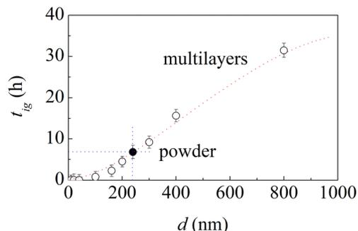
Fig. 4 The ignition time,  $t_{\text{ig}}$ , of multilayers (○) as a function of the bi-layer thickness,  $d$ . The vertical and horizontal dotted lines identify the ignition time of multilayers with  $d$  equal to 240 nm. The ignition time of the pristine Al–Ni powder mixture (●) is also shown. The dotted curve is a guide to the eyes.
