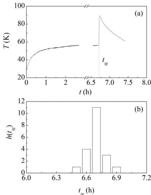
Fig. 1 (a) The typical evolution of the jar temperature due to BM and the mechanochemical ignition of the MSR. (b) The histogram,  $h(t_{ig})$ , of ignition times,  $t_{ig}$ . The histogram has been obtained using 20 independent  $t_{ig}$  estimates.
