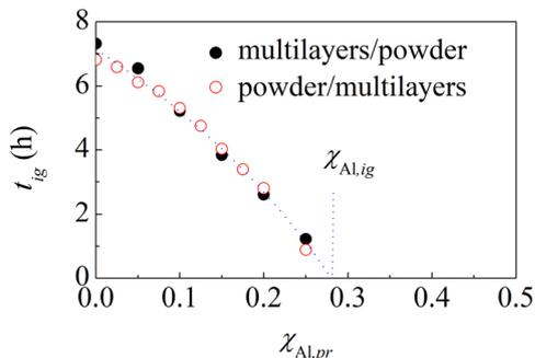
Fig. 8 The ignition time,  $t_{ig}$ , of powder mixtures mixed with multilayers prone to ignition (○) and multilayers mixed with powders prone to ignition (●) as a function of the atomic fraction of Al prone to ignition,  $\chi_{Al,pr}$ . The best-fitted curve is also shown.
