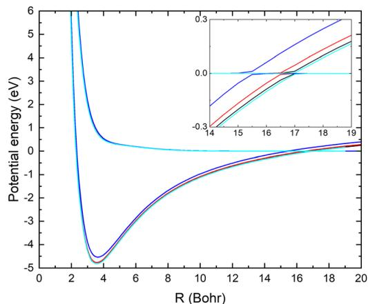
Fig. 1 The two lowest adiabatic potential energy surfaces of LiCN with  $r = 2.22$  bohr and  $\theta = 90^\circ$  calculated with the MRCI method using the aug-cc-pVXZ basis sets, where X = D (red), T (blue), Q (black) and 5 (cyan).
