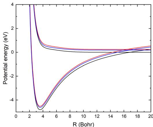
Fig. 5 The two lowest adiabatic potential energy surfaces of LiCN calculated with the MRCI/aug-cc-pVQZ method for  $\theta = 90^\circ$  and  $r = 2.1$  bohr (red), 2.22 bohr (black) and 2.35 bohr (blue).
