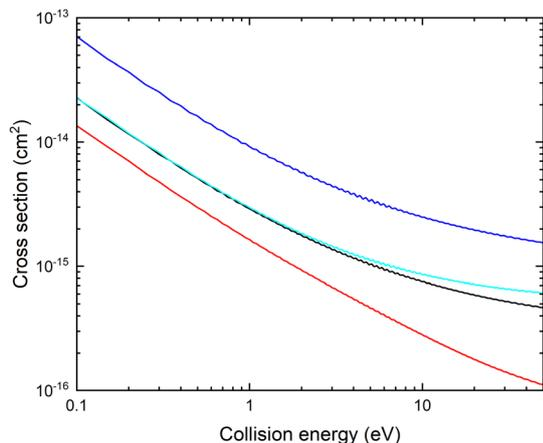
Fig. 3 Fixed  $(r, \theta) = (2.22 \text{ bohr}, 90^\circ)$   $\text{Li}^+ + \text{CN}^-$  mutual neutralization cross section obtained using potentials and couplings computed with MRCI/aug-cc-pVXZ, where X = D (red), T (blue), Q (black) and 5 (cyan).
