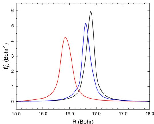
Fig. 6 Non-adiabatic coupling elements  $r_{12}^2$  between the lowest two LiCN states of  $^1A'$  symmetry at fixed  $\theta = 90^\circ$  and  $r = 2.1$  bohr (red), 2.22 bohr (black) and 2.35 bohr (blue).
