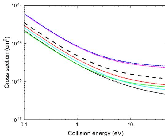
Fig. 7 Cross section  $\sigma(E, r, \theta)$  for mutual neutralization calculated for  $\theta = 90^\circ$  and  $r = 2.1$  bohr (red), 2.17 bohr (cyan), 2.22 bohr (black), 2.25 bohr (green), 2.3 bohr (magenta), 2.35 bohr (blue). The thick black dashed line shows the cross section obtained by averaging over the vibrational motion,  $\bar{\sigma}(E, \theta)$ .
