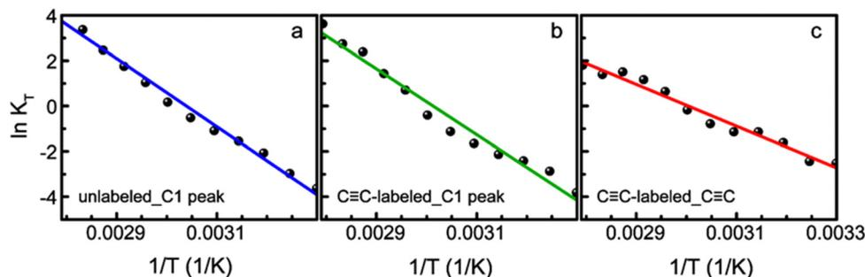
Fig. 4 The van't Hoff plot derived from the C1 band intensity at  $1655\text{ cm}^{-1}$  for the unlabeled strand (a) and the C $\equiv$ C-labeled strand (b), and the C $\equiv$ C stretch band frequency shift for the C $\equiv$ C-labeled strand (c).
