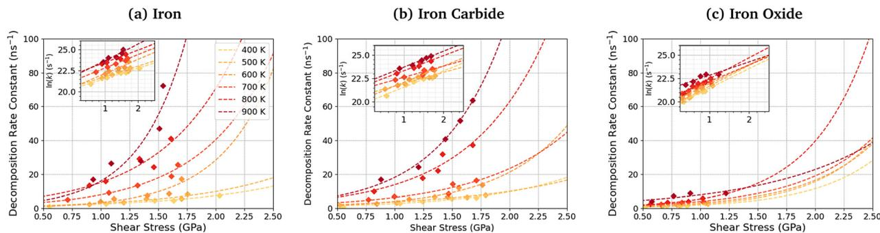
Fig. 11 Shear stress dependence of the TCP decomposition rate at different temperatures for (a)  $\alpha\text{Fe}(110)$ , (b)  $\text{Fe}_3\text{C}(010)$ , and (c)  $\text{Fe}_3\text{O}_4(100)$  systems. Insets show the same data with a logarithmic y-axis.
