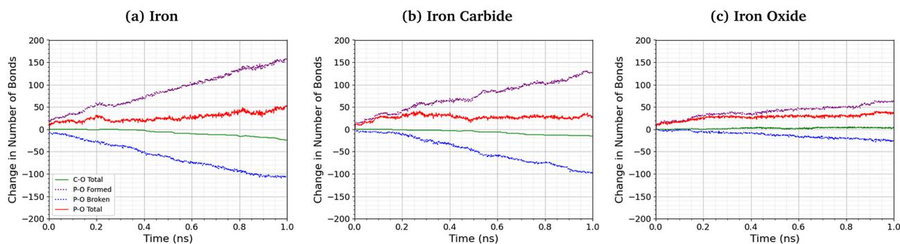
Fig. 8 Change in the number of P–O and C–O bonds with sliding time at 500 K and 3 GPa for the (a)  $\alpha$ -Fe(110), (b)  $\text{Fe}_3\text{C}(010)$ , and (c)  $\text{Fe}_3\text{O}_4(001)$  systems. Solid lines show the change in the total number of bonds compared to TCP, dashed lines show bond formation and dotted lines show bond cleavage.
