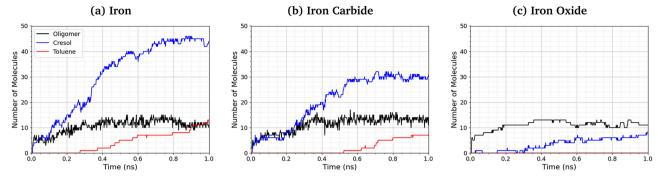
Comparison of oligomer, toluene, and cresol quantities at 500 K and 3 GPa for the (a)  $\alpha$ -Fe(110), (b) Fe<sub>3</sub>C(010), and (c) Fe<sub>3</sub>O<sub>4</sub>(001) systems.
