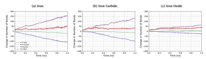
Fig. 8 Change in the number of P-O and C-O bonds with sliding time at 500 K and 3 GPa for the (a) α-Fe(110), (b) Fe<sub>3</sub>C(010), and (c) Fe<sub>3</sub>O<sub>4</sub>(001) systems. Solid lines show the change in the total number of bonds compared to TCP, dashed lines show bond formation and dotted lines show bond cleavage.
