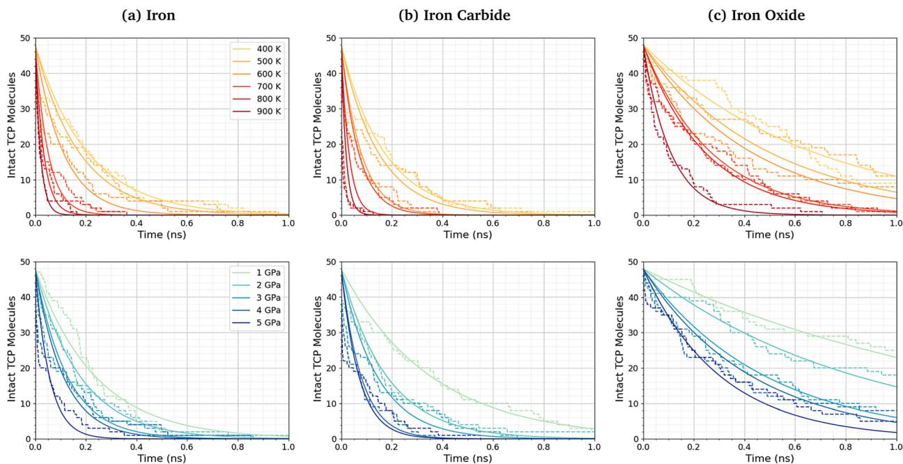
Fig. 5 Number of intact TCP molecules with time at 4 GPa between 400–900 K (top row) and at 600 K between 1–5 GPa (bottom row) for (a)  $\alpha$ -Fe(110), (b)  $\text{Fe}_3\text{C}(010)$ , and (c)  $\text{Fe}_3\text{O}_4(001)$  surfaces. The dashed lines show the simulation data and the solid lines are exponential decay fits used to calculate the first-order rate constants,  $k$ .
