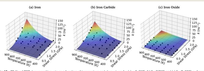
Fig. 13 3D fits of TCP decomposition rate as a function of temperature and shear stress for (a)  $\alpha$ -Fe(110), (b) Fe<sub>3</sub>C(010) and (c) Fe<sub>3</sub>O<sub>4</sub>(100) surfaces.
