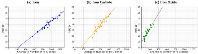
Variation in ln(k) for TCP decomposition with the change in the number of Fe-C bonds from 0-1 ns for (a) α-Fe(110), (b) Fe<sub>3</sub>C(010), and (c) Fe<sub>3</sub>O<sub>4</sub>(100).
