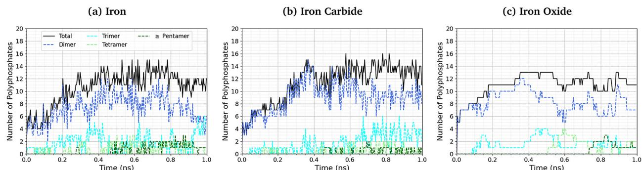
Fig. 10 Change in the number of polyphosphate chains with sliding time at 500 K and 3 GPa for (a)  $\alpha$ -Fe(110), (b)  $\text{Fe}_3\text{C}(010)$  and (c)  $\text{Fe}_3\text{O}_4(100)$  systems.
