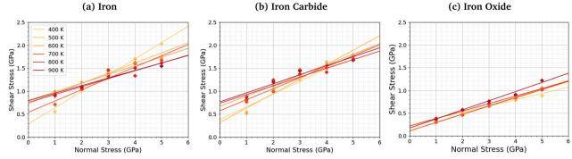
Variation in shear stress with changes in normal stress for (a)  $\alpha$ -Fe(110), (b) Fe<sub>3</sub>C(010), and (c) Fe<sub>3</sub>O<sub>4</sub> (001) surfaces
