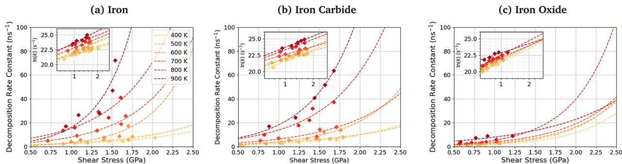
Fig. 11 Shear stress dependence of the TCP decomposition rate at different temperatures for (a)  $\alpha$ -Fe(110), (b)  $\text{Fe}_3\text{C}(010)$ , and (c)  $\text{Fe}_3\text{O}_4(100)$  systems. Insets show the same data with a logarithmic y-axis.
