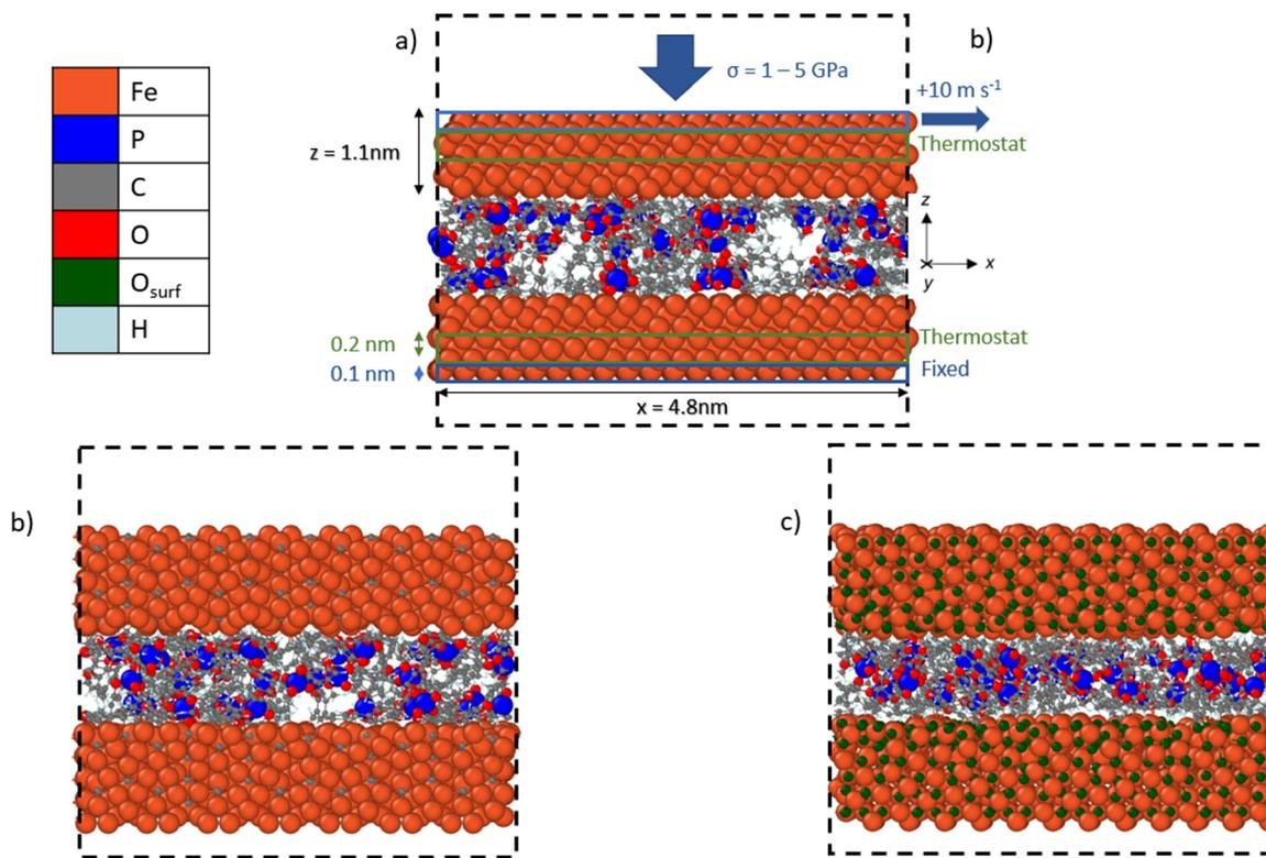
Fig. 2 Side-view snapshots showing the model systems with TCP molecules confined between (a)  $\alpha$ -Fe(110), (b)  $\text{Fe}_3\text{C}(010)$ , and (c)  $\text{Fe}_3\text{O}_4(001)$ -SCV surfaces. Systems shown after minimisation and equilibration, but before heating, compression, and shear. Black dashed line shows the simulation box. Rendered using OVITO.<sup>42</sup>
