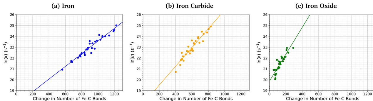
Fig. 7 Variation in  $\ln(k)$  for TCP decomposition with the change in the number of Fe-C bonds from 0–1 ns for (a)  $\alpha$ -Fe(110), (b)  $\text{Fe}_3\text{C}(010)$ , and (c)  $\text{Fe}_3\text{O}_4(100)$ .
