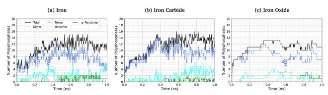
Fig. 10 Change in the number of polyphosphate chains with sliding time at 500 K and 3 GPa for (a)  $\alpha$ -Fe(110), (b) Fe<sub>3</sub>C(010) and (c) Fe<sub>3</sub>O<sub>4</sub>(100) systems.
