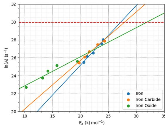
Fig. 12 Kinetic compensation effect between the activation energy and pre-exponential factor for iron, iron carbide, and iron oxide.
