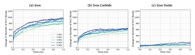
Fig. 6 Change in the number of Fe-C bonds with simulation time at 600 K between 1-5 GPa for (a) α-Fe(110), (b) Fe<sub>3</sub>C(010), and (c) Fe<sub>3</sub>O<sub>4</sub>(100).
