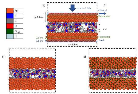
Fig. 2 Side-view snapshots showing the model systems with TCP molecules confined between (a) α-Fe(110), (b) Fe<sub>3</sub>C(010), and (c) Fe<sub>3</sub>O<sub>4</sub>(001)-SCV surfaces. Systems shown after minimisation and equilibration, but before heating, compression, and shear. Black dashed line shows the simulation box. Rendered using OVITO.42
