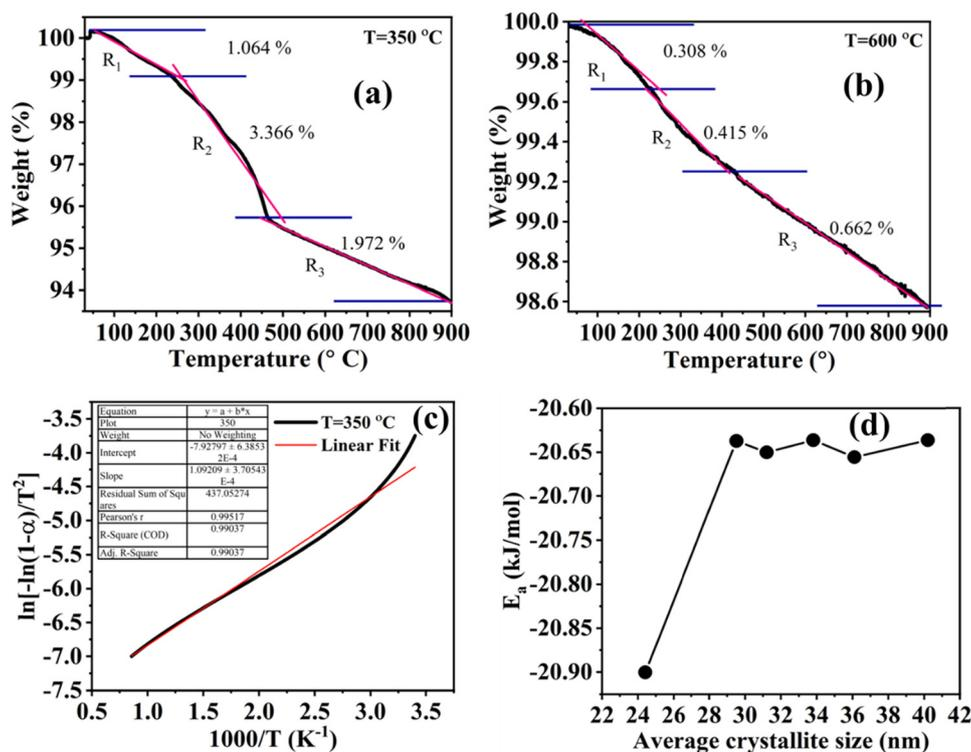
Fig. 6 Thermogravimetry (TGA) plot for BiFeO<sub>3</sub> nanoparticle samples annealed at (a) 350 °C and (b) 600 °C, (c) linear fitting curve of the  $\ln[-\ln(1-\alpha)]$  versus  $\frac{1000}{T}$  graph for  $T_{\text{Calcination}} = 350$  °C BFO NPs to calculate the activation energy and (d) variation of the activation energy w.r.t average crystallite size.
