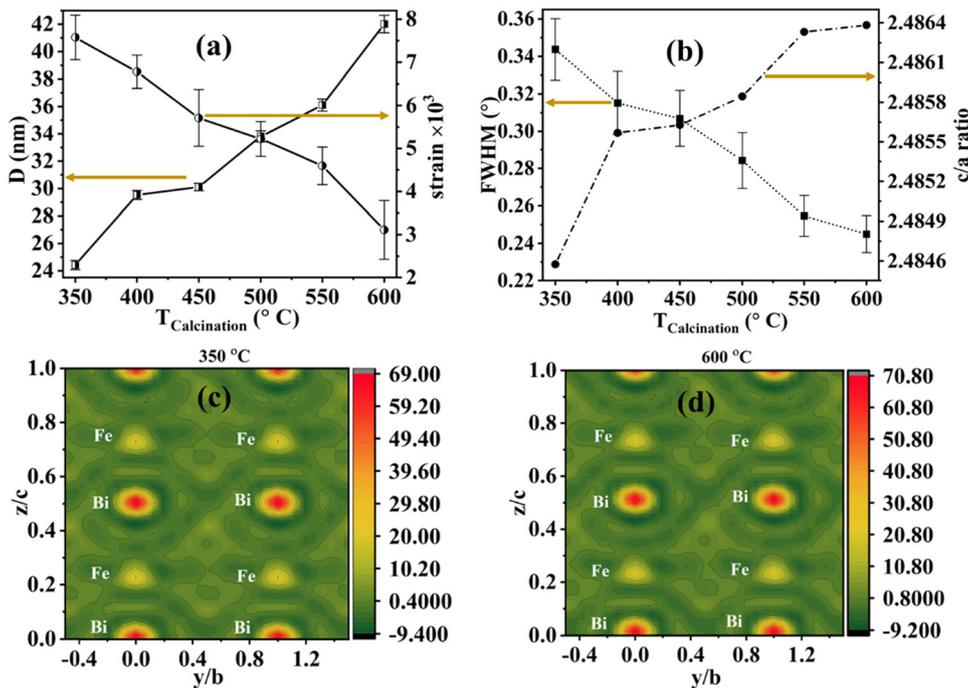
Fig. 3 Variation of (a) average crystallite size and lattice strain, (b) FWHM of the (104) plane, and the  $c/a$  ratio of  $\text{BiFeO}_3$  nanoparticles w.r.t. different calcination temperatures. (c and d) The electron density plots for  $\text{BiFeO}_3$  nanoparticles calcined at different temperatures – 350 °C, and 600 °C, plotted in the  $yz$  plane at  $x$  intercept = 0.
