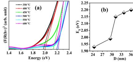
Fig. 10 (a) Tauc plot to estimate the direct band gap and (b) the variation of optical band gap with average particle size for different annealed  $BiFeO_3$  nanoparticle samples.
