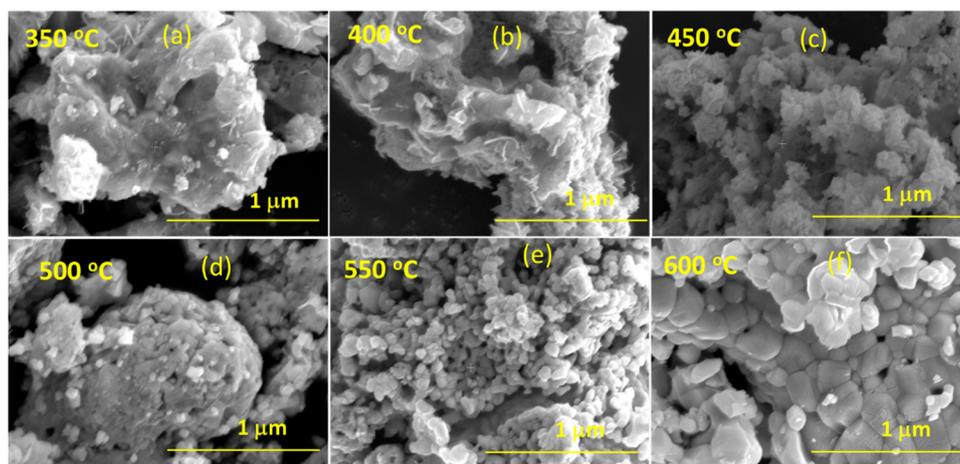
Fig. 4 Scanning electron microscope image of  $\text{BiFeO}_3$  nanoparticles annealed at  $T_{\text{Calcination}}$  (a) 350 °C, (b) 400 °C, (c) 450 °C, (d) 500 °C, (e) 550 °C, and (f) 600 °C.
