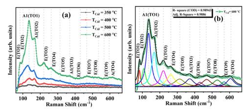
Fig. 8 Room temperature Raman spectra of BiFeO $_3$  nanoparticles annealed at (a) 350, 400, 500 and 600 °C (b) with possible peaks fitted to show the Raman modes in the 600 °C annealed sample, clearly showing all 13 Raman modes.
