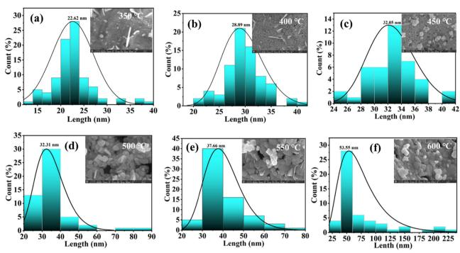
Fig. 5 (a-f) Grain size distribution plots for different annealed  $BiFeO_3$  nanoparticle samples, showing the average grain size with the inset showing the respective FESEM images.
