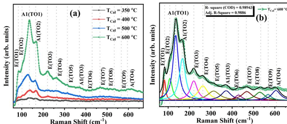
Fig. 8 Room temperature Raman spectra of BiFeO<sub>3</sub> nanoparticles annealed at (a) 350, 400, 500 and 600 °C (b) with possible peaks fitted to show the Raman modes in the 600 °C annealed sample, clearly showing all 13 Raman modes.
