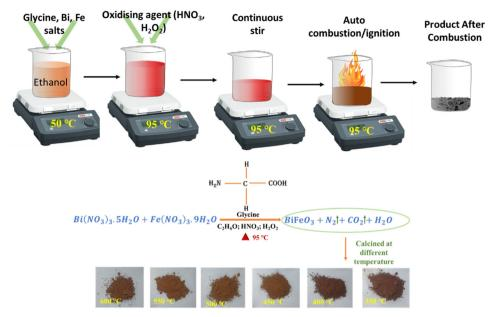
Fig. 1 Schematic presentation of the synthesis process and chemical reaction for BiFeO<sub>3</sub> nanoparticles using the auto combustion method and the optical images of different temperature annealed BFO nanoparticles.
