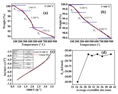
Fig. 6 Thermogravimetry (TGA) plot for BiFeO $_3$  nanoparticle samples annealed at (a) 350 °C and (b) 600 °C, (c) linear fitting curve of the  $\log\left[\frac{-\log(1-\alpha)}{T^2}\right]$  versus  $\frac{1000}{T}$  graph for  $T_{\text{Calcination}}$  = 350 °C BFO NPs to calculate the activation energy and (d) variation of the activation energy w.r.t average crystallite size.
