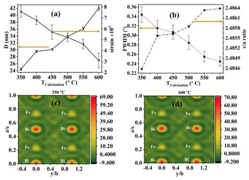
Fig. 3 Variation of (a) average crystallite size and lattice strain, (b) FWHM of the (104) plane, and the c/a ratio of BiFeO<sub>3</sub> nanoparticles w.r.t. different calcination temperatures. (c and d) The electron density plots for BiFeO<sub>3</sub> nanoparticles calcined at different temperatures – 350 °C, and 600 °C, plotted in the yz plane at x intercept = 0.
