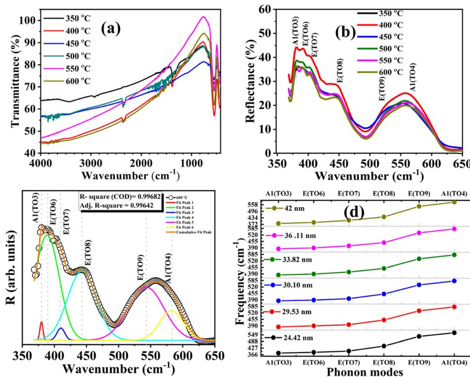
Fig. 7 (a) Fourier transform infrared spectroscopy spectra in transmittance mode and (b) reflectance plot for the variation of  $R$  (%) with wavenumber for different annealed BFO-NPs, (c) fitted plot of reflectance vs. wavenumber for BFO-NPs annealed at 600 °C, where the presence of different IR phonon modes is mentioned, and (d) plot for variation of different IR phonon modes with increasing average crystallite size.
