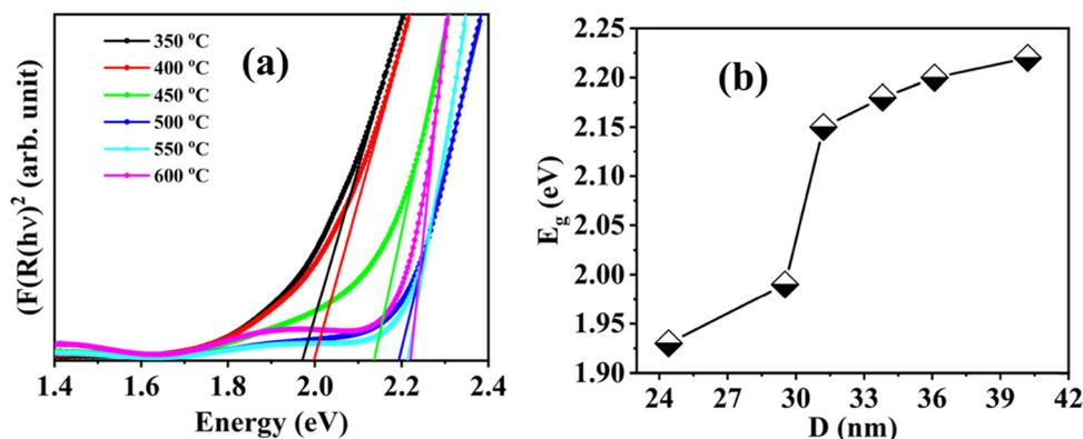
**Fig. 10** (a) Tauc plot to estimate the direct band gap and (b) the variation of optical band gap with average particle size for different annealed BiFeO<sub>3</sub> nanoparticle samples.
