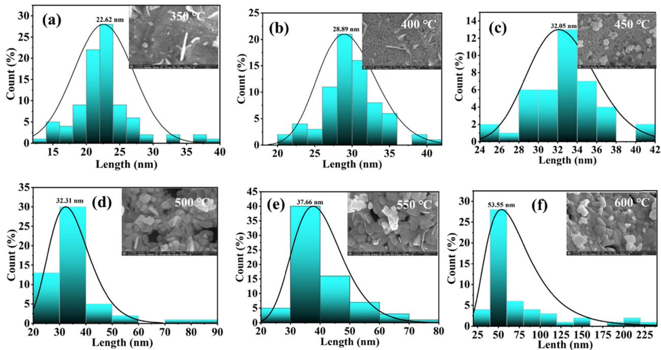
Fig. 5 (a–f) Grain size distribution plots for different annealed BiFeO<sub>3</sub> nanoparticle samples, showing the average grain size with the inset showing the respective FESEM images.
