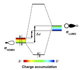
Fig. 4 A larger accumulation of negative charge  $(\delta^-)$  destabilizes the occupied molecular orbitals ( $\sigma_{\rm HOMOs}\!)$  of H-bond acceptors, while a larger accumulation of positive charge  $(\delta^+)$  stabilizes the unoccupied molecular orbitals ( $\sigma_{LUMOs}$ ) of H-bond donors. This results in a smaller HOMO-LUMO energy gap ( $\Delta \varepsilon$ ) and therefore a better  $\sigma$ -orbital interaction in case of enhanced charge accumulation
