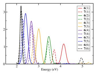
Fig. 3 Theoretical absorbance spectra of molecules 6(n) and 7(n) with n = 11 to 6 in the gas phase at the TD-DFT/B3LYP/TZP level with 5 excited states
