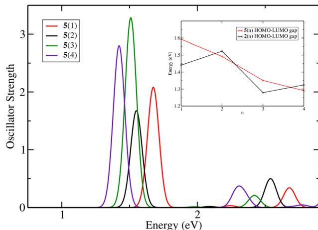
Fig. 5 Theoretical absorbance spectra of molecules  $5(n)$  with  $n = 1$  to 4 in the gas phase at the TD-DFT/B3LYP/TZP level with 5 excited states. The inset graph shows a comparison between the HOMO–LUMO gap for  $2(n)$  and  $5(n)$ .
