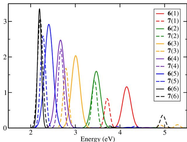
Fig. 3 Theoretical absorbance spectra of molecules  $6(n)$  and  $7(n)$  with  $n = 1$  to 6 in the gas phase at the TD-DFT/B3LYP/TZP level with 5 excited states.
