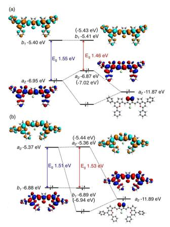
Saturated ring analysis of molecules 2(n): n = 1 (a) and n = 2 (b), NBO study excluding interaction between C<sub>2</sub>H<sub>4</sub> and the polymethine chain. The orbital energies of the molecules without the C2H4 moiety (5(n)) are presented in brackets. HOMOs are presented in blue-red and the LUMOs are presented in cyan-orange. The colour difference in the molecular orbitals indicates a difference in sign
