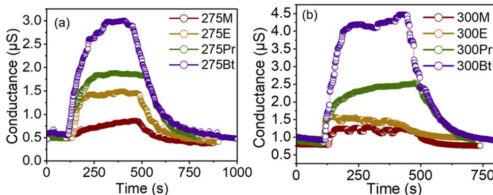
Fig. 6 Comparison among the sensing responses towards methanol, ethanol, propanol, and butanol vapours at (a) 275 °C and (b) 300 °C.
