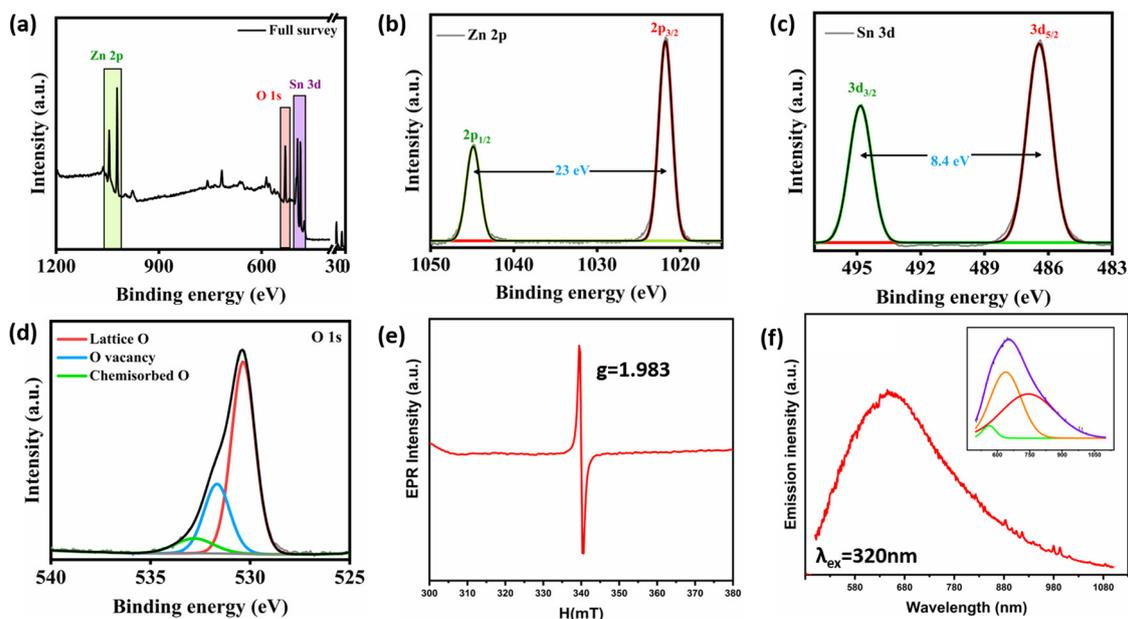
Fig. 2 (a) XPS survey scan, core level spectra of: (b) Zn 2p, (c) Sn 3d, (d) O 1s; (e) EPR spectrum; and (f) photoluminescence spectrum of Zn<sub>2</sub>SnO<sub>4</sub>.
