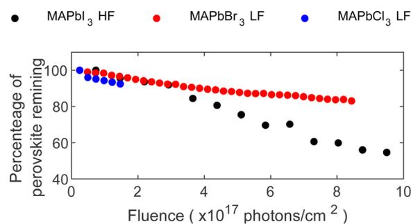
**Fig. 6** Percentage of perovskite remaining at the surface as function of X-ray fluence ( $\text{photons cm}^{-2}$ ). Determined by the percentage of  $\text{N}^+/\Sigma\text{Pb}$  in  $\text{MAPbI}_3$  and the percentage of  $\text{Pb}^{2+}/\Sigma\text{Pb}$  in  $\text{MAPbBr}_3$  and  $\text{MAPbCl}_3$ .
