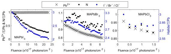
Fig. 3 Core level intensity evolution for the crystal surfaces of MAPbl<sub>x</sub> (left), MAPbBr<sub>x</sub> (middle) and MAPbCl<sub>x</sub> (right) as a function of the fluence (photons cm<sup>-2</sup>). Intensity normalized by the total amount of lead (Pb<sup>0</sup> + Pb<sup>2+</sup>) and initial ratios set to those expected from the perovskite stoichiometry (1 nitrogen and 3 halides). The left axes (black) refer to Pb2+ and N, the right axes (blue) refer to the halide
