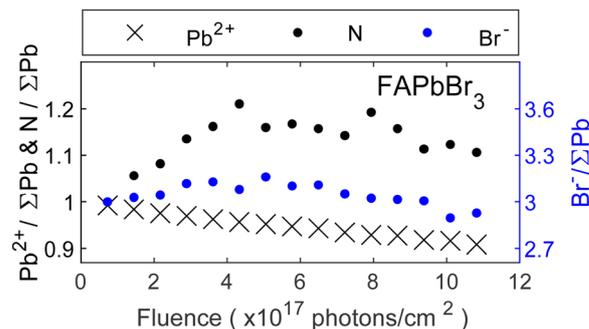
Fig. 4 Core level intensity evolution for the  $\text{FAPbBr}_3$  crystal surface as a function of fluence (photons  $\text{cm}^{-2}$ ). Intensity normalized by the total amount of lead ( $\text{Pb}^0 + \text{Pb}^{2+}$ ) and initial ratios set to those expected from the perovskite stoichiometry (1 cation represented by nitrogen and 3 bromide).
