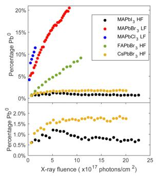
Fig. 2 Percentage Pb<sup>0</sup> (Pb<sup>0</sup> intensity/total Pb intensity) on the surface of each material (MAPbI<sub>3</sub>, MAPbBr<sub>3</sub>, MAPbCl<sub>3</sub>, FAPbBr<sub>3</sub>, CsPbBr<sub>3</sub>) as a function of fluence (photons cm<sup>-2</sup>). Top panel: All compositions. Bottom panel: Zoom on MAPbl<sub>3</sub> and CsPbBr<sub>3</sub>.
