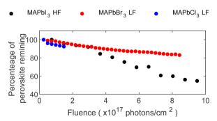
Fig. 6 Percentage of perovskite remaining at the surface as function of Xray fluence (photons cm<sup>-2</sup>). Determined by the percentage of N<sup>+</sup>/ $\sum$ Pb in MAPbl<sub>3</sub> and the percentage of Pb<sup>2+</sup>/∑Pb in MAPbBr<sub>3</sub> and MAPbCl<sub>3</sub>.
