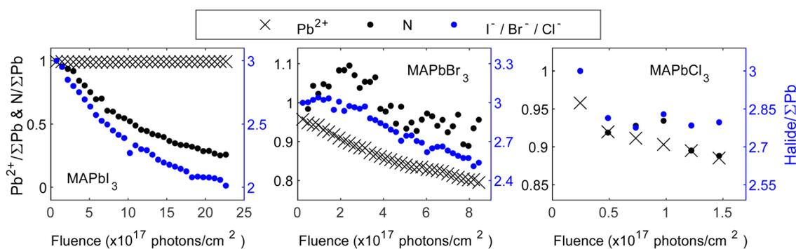
Fig. 3 Core level intensity evolution for the crystal surfaces of MAPbI<sub>3</sub> (left), MAPbBr<sub>3</sub> (middle) and MAPbCl<sub>3</sub> (right) as a function of the fluence (photons cm<sup>-2</sup>). Intensity normalized by the total amount of lead (Pb<sup>0</sup> + Pb<sup>2+</sup>) and initial ratios set to those expected from the perovskite stoichiometry (1 nitrogen and 3 halides). The left axes (black) refer to Pb<sup>2+</sup> and N, the right axes (blue) refer to the halide.
