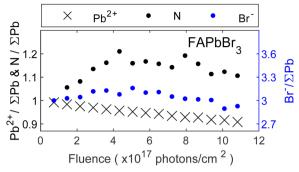
Fig. 4 Core level intensity evolution for the FAPbBr<sub>3</sub> crystal surface as a function of fluence (photons cm<sup>-2</sup>). Intensity normalized by the total amount of lead (Pb<sup>0</sup> + Pb<sup>2+</sup>) and initial ratios set to those expected from the perovskite stoichiometry (1 cation represented by nitrogen and 3 bromide).
