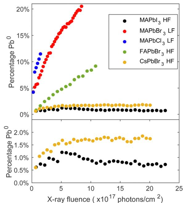
Fig. 2 Percentage Pb<sup>0</sup> (Pb<sup>0</sup> intensity/total Pb intensity) on the surface of each material (MAPbI<sub>3</sub>, MAPbBr<sub>3</sub>, MAPbCl<sub>3</sub>, FAPbBr<sub>3</sub>, CsPbBr<sub>3</sub>) as a function of fluence (photons cm<sup>-2</sup>). Top panel: All compositions. Bottom panel: Zoom on MAPbI<sub>3</sub> and CsPbBr<sub>3</sub>.
