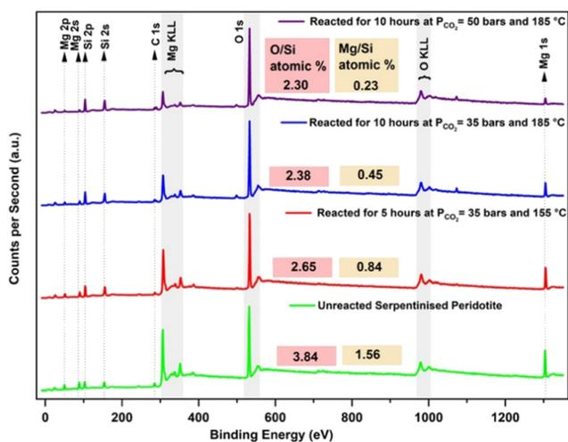
Fig. 4 Evidence of changes in the chemical composition of serpentinized peridotite when reacted in 0.1 M  $\text{Na}_2\text{H}_2\text{EDTA}\cdot 2\text{H}_2\text{O}$  chelating agent and 2 M  $\text{NaHCO}_3$  and a stirring speed of 500 rpm based on X-ray photoelectron spectroscopy (XPS) measurements. The peaks corresponding to C 1s, O 1s, Si 2p, Mg 1s, Mg 2p core levels and the Auger structure (O KLL, Mg KLL) are indicated.
