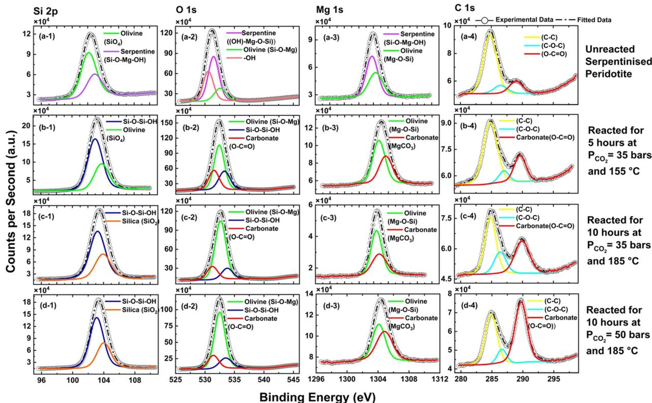
Fig. 5 Identification of changes in the chemical states of silicon (a-1)–(d-1), oxygen (a-2)–(d-2), magnesium (a-3)–(d-3) and carbon (a-4)–(d-4) via deconvolution of Si 2p, O 1s, Mg 1s, and C 1s peaks in the unreacted and reacted serpentinized peridotite reacted under various experimental conditions.
