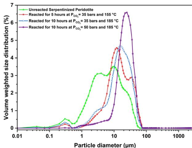
Fig. 6 Particle size distribution of serpentinized peridotite when reacted with  $\text{CO}_2$  under different reaction conditions using 0.1 M  $\text{Na}_2\text{H}_2\text{EDTA}\cdot 2\text{H}_2\text{O}$  chelating agent and 2 M  $\text{NaHCO}_3$ , slurry density of 15 wt% and a stirring speed of 500 rpm.
