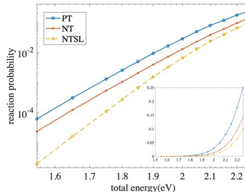
Fig. 2 Nonadiabatic tunneling probability against energy. PT: optimized pure tunneling through  $E_1(r,R)$ , NT: optimized nonadiabatic tunneling, NTSL: nonadiabatic tunneling along a straight line. The saddle point energy of the lower adiabatic potential is  $E_{\text{sp}} = 2.275$  eV.
