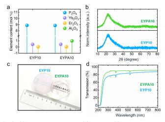
Fig. 2 (a) Measured compositions, (b) XRD data, (c) real photographs of EYP10 and EYPA10 glasses, and (d) transmittance curves in the ultravioletvisible spectral range (200-800 nm) for EYP10 and EYPA10 glasses.
