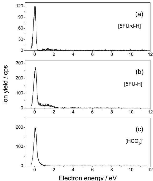
Fig. 2 Yield function of the (a) dehydrogenated parent anion  $[5\text{FUrd-H}]^-$ , (b) dehydrogenated 5-fluorouracil anion  $[5\text{FU-H}]^-$  produced from the *N*-glycosidic bond cleavage, and (c)  $[\text{HCO}_2]^-$  anion.
