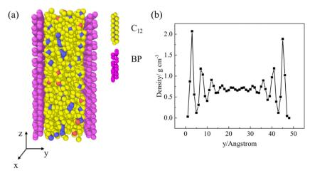
Fig. 1 (a) Schematic of the simulation setup in which C<sub>12</sub> molecules are confined in a BP nanochannel which the blue and red atoms represented the middle carbon atoms and head/tail carbon atoms. (b) The density distribution of C<sub>12</sub> along the y-axis.
