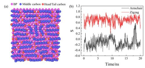
Fig. 4 (a) x-z cross-sectional view of the one-layered structure, in which the molecular chains of C<sub>12</sub> are aligned parallel to the BP wall. (b) The orientation parameter S value versus time along armchair and zigzag directions in 2-nm BP nanochannels.
