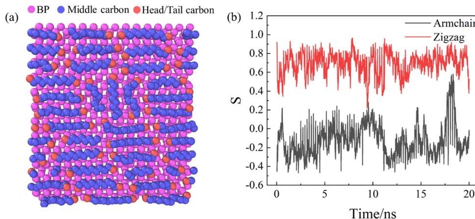
Fig. 4 (a)  $x$ - $z$  cross-sectional view of the one-layered structure, in which the molecular chains of  $C_{12}$  are aligned parallel to the BP wall. (b) The orientation parameter  $S$  value versus time along armchair and zigzag directions in 2-nm BP nanochannels.
