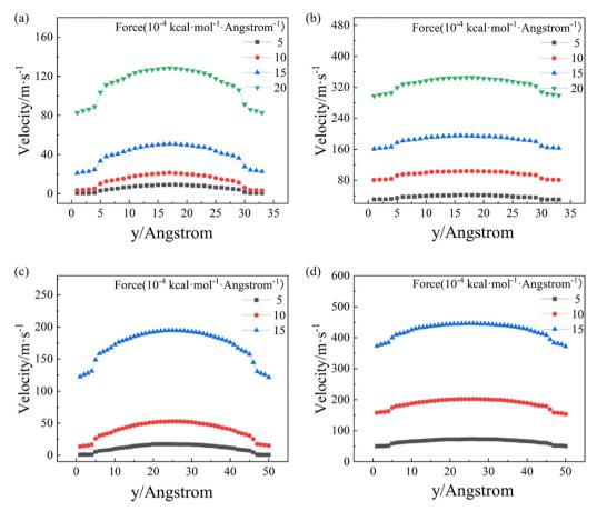
Fig. 5 Velocity profiles of the  $C_{12}$  molecules confined in 4-nm BP nanochannels when flowing along the (a) armchair direction and (b) zigzag direction. Velocity profiles of the  $C_{12}$  molecules confined in 6-nm BP nanochannels when flowing along the (c) armchair direction and (d) zigzag direction.
