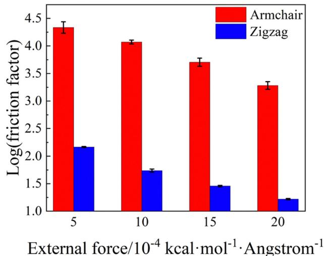
Fig. 3 The logarithm of the friction factor between  $C_{12}$  molecules and BP nanochannels under external driving forces ranging from  $5 \times 10^{-4}$  to  $2 \times 10^{-3} \text{ kcal mol}^{-1} \text{ \AA}^{-1}$ .
