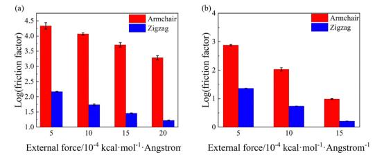
Fig. 6 The logarithm of the friction factor between C<sub>12</sub> molecules and BP nanochannels for BP nanochannels with widths of (a) 4 nm and (b) 6 nm.
