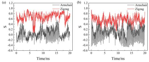
S values of one-layered C<sub>12</sub> molecules close to the BP wall along the armchair and zigzag directions in (a) 4-nm and (b) 6-nm nanochannels.
