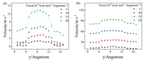
Fig. 2 Velocity profiles of the C<sub>12</sub> molecules flowing along the (a) armchair direction and (b) zigzag direction under different external driving forces in a 2-nm BP nanochannel.
