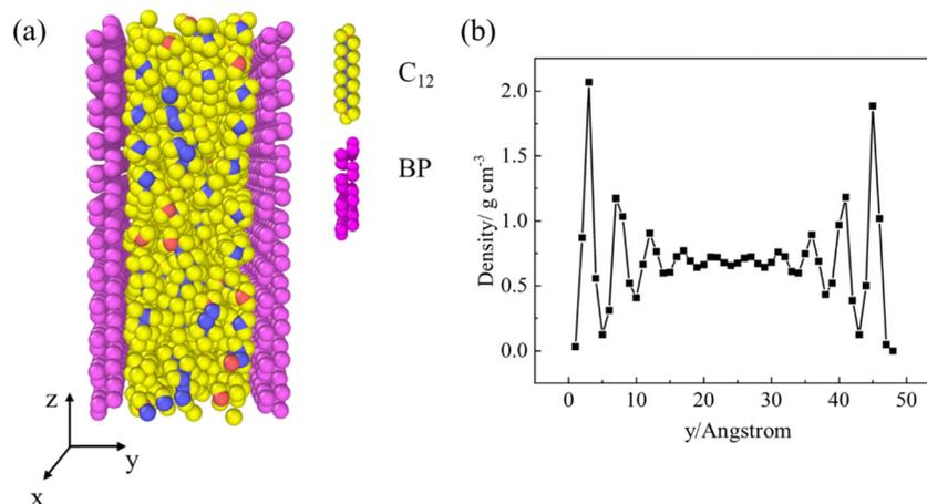
Fig. 1 (a) Schematic of the simulation setup in which  $C_{12}$  molecules are confined in a BP nanochannel which the blue and red atoms represented the middle carbon atoms and head/tail carbon atoms. (b) The density distribution of  $C_{12}$  along the  $y$ -axis.
