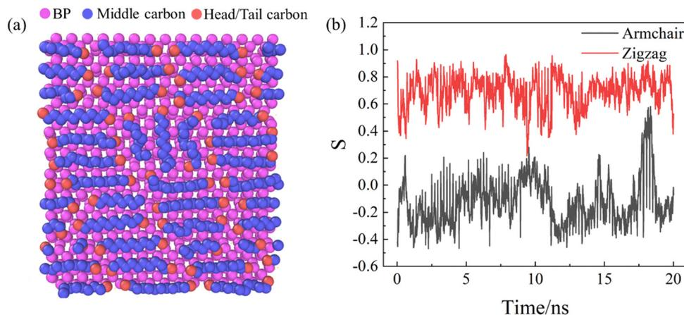
Fig. 4 (a)  $x$ - $z$  cross-sectional view of the one-layered structure, in which the molecular chains of  $C_{12}$  are aligned parallel to the BP wall. (b) The orientation parameter  $S$  value versus time along armchair and zigzag directions in 2-nm BP nanochannels.
