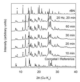
Fig. 2 XRPD data of rBN/BQ ball milled at a 1:1 mole ratio shown in comparison to the reference powder data calculated from the published crystal structure of cocrystal I and the experimental powder data of rBN. Ball milling was done for different times at 25 Hz except for the one sample indicated in the figure. 480-490 mg of total solids were used for the experiments. The peaks marked with "\*" at 8° and 11.1°  $2\theta$  are associated with unreacted rBN.
