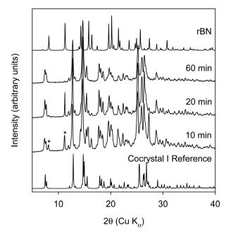
Fig. 3 XRPD data of rBN/BQ ball milled at a 1:1.5 mole ratio shown in comparison to the reference powder data calculated from the published crystal structure of cocrystal I and the experimental powder data of rBN. Ball milling was done for different times at 25 Hz. 570 mg of total solids were used for the experiment. The peaks marked with "\*" at  $8^{\circ}$  and  $11.1^{\circ}$   $2\theta$ are associated with unreacted rBN.
