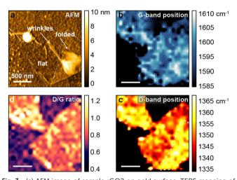
Fig. 3 (a) AFM image of sample rGO2 on gold surface. TERS mapping of the region in (a) based on (b) the G-band position, (c) D-band position, and (d)  $I_D/I_G$  ratio
