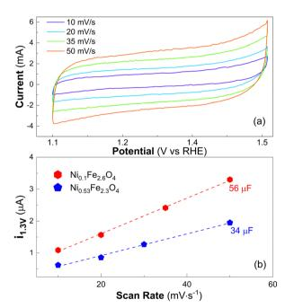
Fig. 5 (a) CV at different scan rates on Ni<sub>0.1</sub>Fe<sub>2.6</sub>O<sub>4</sub> and relative linear fit of the current at 1.3 V vs. RHE (b). The obtained values of double layer capacitance are reported on the graph with corresponding colors.
