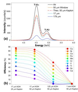
Fig. 4 (a) Ti  $K\alpha$  and  $K\beta$  acquired ex situ (air), with Kapton window and for two different liquid layer thickness, compared with the theoretical transmittance of 50 µm of Kapton; 35 (b) theoretical efficiency of the cell for various elements, calculated for different electrolyte (KOH 0.1 M) and window thickness, assuming a probing energy 200 eV above the K absorption edge and the relative Kα line as outgoing energy.
