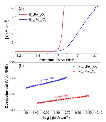
Fig. 6  $\,$  iR corrected LSV (a) with relative Tafel plot slopes (b). The noise above 10 mA cm $^{-2}$  is due to the formation of oxygen bubbles.
