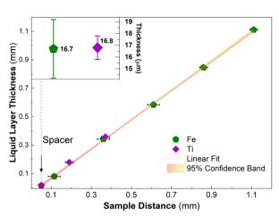
Fig. 3 Liquid layer thickness vs. sample-spacer distance. The linear fit  $(R^2 = 0.999)$  was carried out on the data acquired from the Fe foil (green) and confronted with the result obtained from Ti (purple). In the inset, the minimal thickness estimated from the two measurements.
