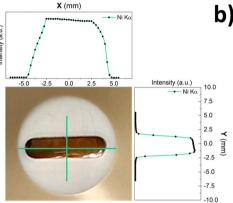
Fig. 2 (a) Electrochemical cell mounted at SAMBA beamline; (b) inset of the cell window with the liquid layer profile curves
