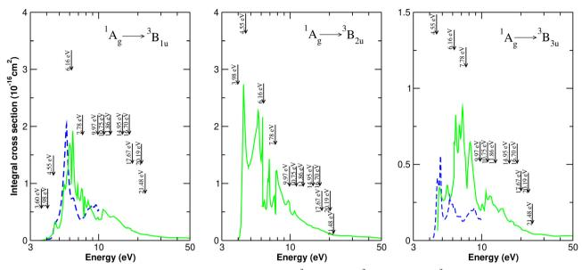
Fig. 7 Integral cross sections for the excitation from the ground state to the  $1^3B_{1u}$  (3.60 eV),  $1^3B_{2u}$  (3.98 eV) and  $1^3B_{3u}$  (4.55 eV) excited states of pyrazine by electron impact. Solid green line, present SMCPP results; dashed blue line, R-matrix results from Mašín and Gorfinkiel.<sup>6</sup>
