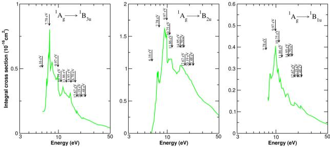
Fig. 8 Integral cross sections for the excitation from the ground state to the  $1^{1}B_{3u}$  (5.39 eV),  $1^{1}B_{2u}$  (6.16 eV) and  $1^{1}B_{1u}$  (7.28 eV) excited states of pyrazine by electron impact. Solid green line, present SMCPP results.
