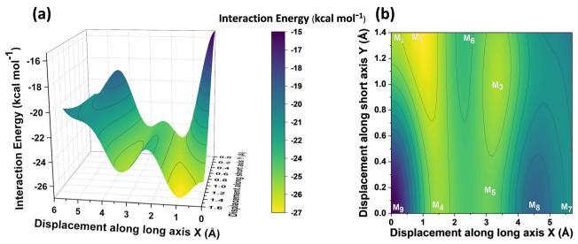
Fig. 4 (a) PES of PDI dimer showing interaction energy as a function of displacement along long axis X and short axis Y. (b) 2-D contour plot showing the stationary points on the PES. Step size for displacement = 0.1 Å.
