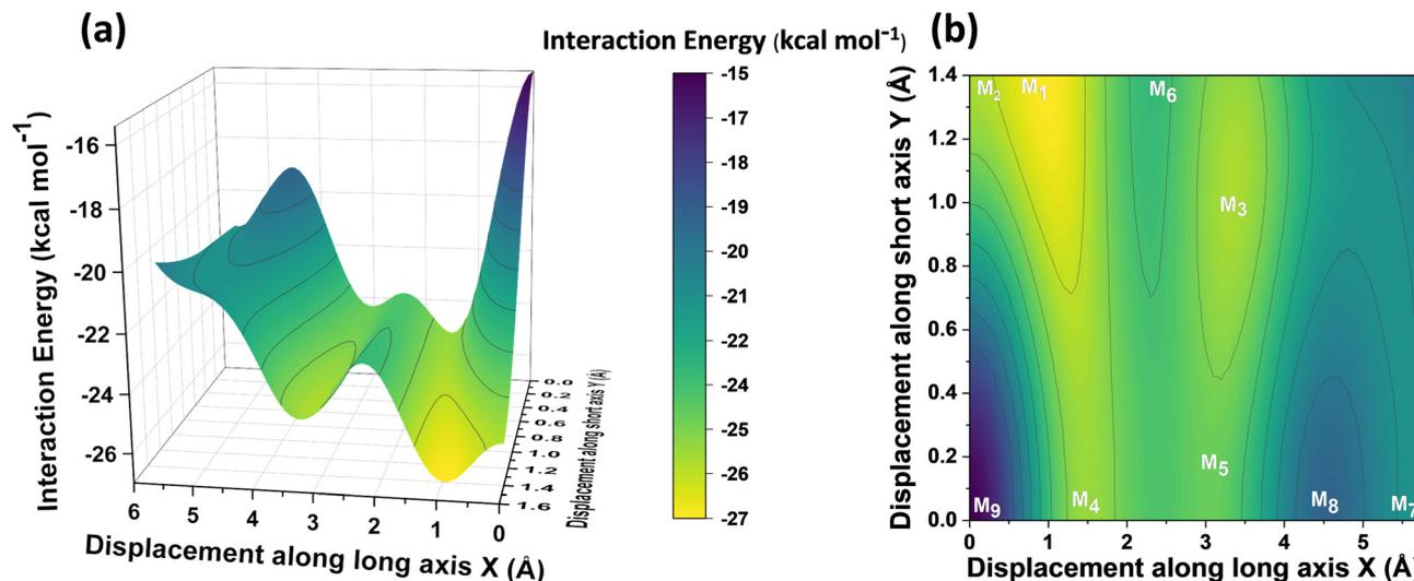
Fig. 4 (a) PES of PDI dimer showing interaction energy as a function of displacement along long axis  $X$  and short axis  $Y$ . (b) 2-D contour plot showing the stationary points on the PES. Step size for displacement = 0.1 Å.
