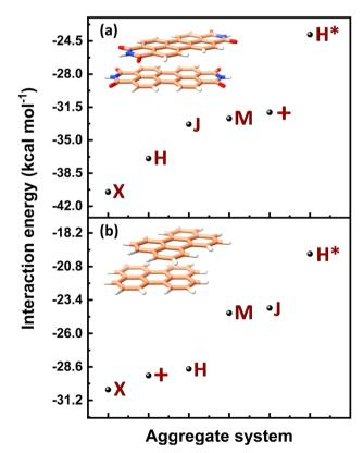
Fig. 8 Interaction energy profiles of different dimer systems of (a) PDI and (b) perylene aggregate systems computed through SAPT.
