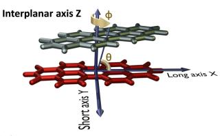
Fig. 2 Dimer model of the perylenediimide chromophore showing axes labels, rotation angle  $(\phi)$  and slip angle  $(\theta)$ .
