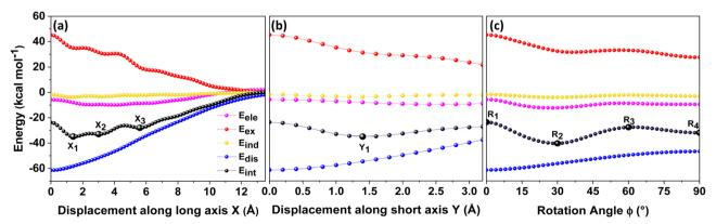
Fig. 3 Variation of the total interaction energy ( $E_{int}$ ) and the components; electrostatics ( $E_{ele}$ ), exchange ( $E_{ex}$ ), induction ( $E_{ind}$ ), and dispersion ( $E_{dis}$ ) computed through SAPT as a function of (a) displacement along long axis X, (b) displacement along short axis Y and (c) rotation about the interplanar axis Z in PDI dimer.
