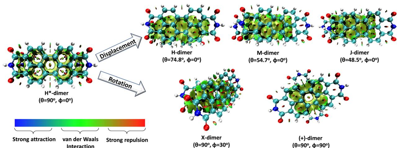
Fig. 6 NCI isosurfaces (isovalue = 0.5 a.u.) showing non-covalent interactions in different types of PDI dimer systems. Green surfaces and red surfaces represent stabilizing and destabilizing interactions, respectively.
