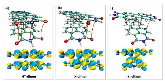
Fig. 7 QTAIM plots (top) showing the BCPs between the monomers and HOMO isosurfaces (isovalue = 0.017 a.u.) (bottom) showing the interactions between the orbital lobes of the two monomers in (a) H\*-, (b) X- and (c) (+)-dimers of PDI.
