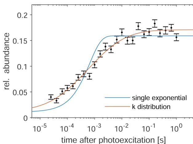
Fig. 3 Relative fragment yield of  $\text{Sn}_{15}^-$  as a function of delay time for 500 nm photon wavelength. The blue and yellow lines are fits of a single exponential function and of a distribution of such functions, respectively, to the data. For details, see the main text.
