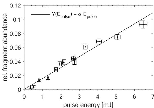
Fig. 2 Relative yield of the  $\text{Sn}_{15}^-$  fragment as a function of excitation-pulse energy at 532 nm. The horizontal and vertical error bars show the shot-to-shot noise of the laser and the statistical uncertainty of the ion signal, respectively. The solid line is a linear fit.
