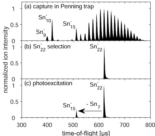
Fig. 1 Time-of-flight spectra (each normalized to its highest signal) of tin clusters (a) after their capture and buffer-gas cooling of the ion motion, (b) after mass selection of  $\text{Sn}_{22}^-$ , and (c) after photoexcitation with 2.48 eV photons and ion ejection after a delay of one second.
