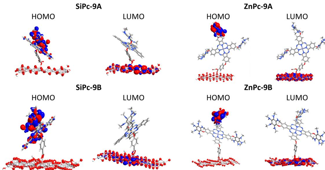
Fig. 7 Surfaces of the frontier molecular orbitals calculated for the interaction dye-TiO<sub>2</sub> with an anhydrous group (top) and a carboxyl group (bottom).
