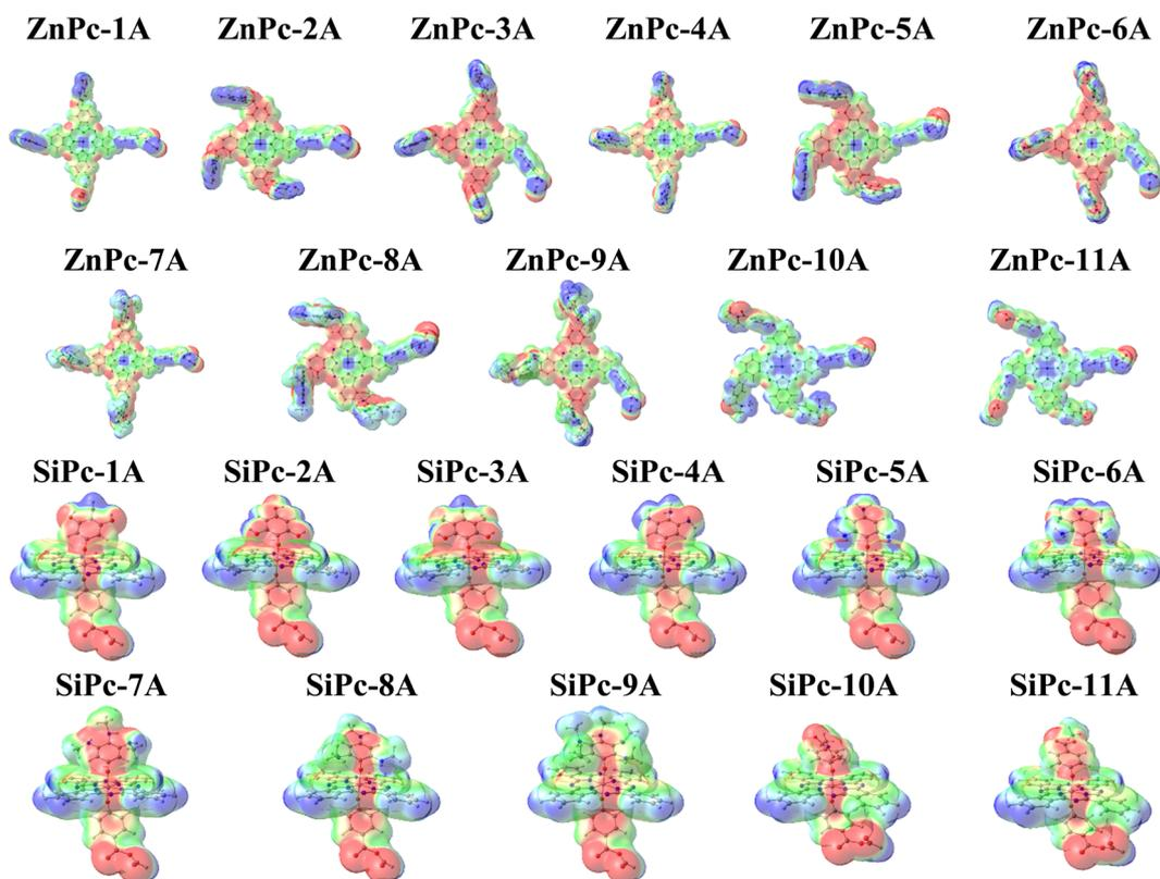
Fig. 3 Surfaces of molecular electrostatic potential mapped into the charge density isosurface of 0.002 electrons per Bohr<sup>3</sup> for both MPcs with anhydrous as the anchoring group.
