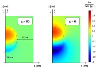
Fig. 3 Normalized electrostatic potential  $\Psi_{\varepsilon}$  distribution of immersed in an empty medium characterized by different dielectric constants: on the left  $\varepsilon_r$  = 80; on the right  $\varepsilon_r$  = 6
