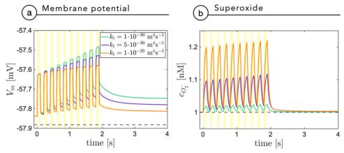
Fig. 7 The membrane potential (a) and the superoxide concentration (b) are shown as a function of time secondary to a train of light stimuli with an on/ off duty cycle of 100 ms. The results are reported for three different values of the tunneling coefficient  $k_{tr}$ , normally assumed equal to  $10^{-30}$  m<sup>4</sup> s<sup>-1</sup>, in agreement with the study by Rudolph et al. 28
