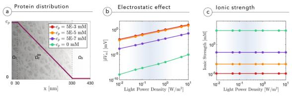
Fig. 4 (a) Cleft proteinic distribution across the electrolytic domain, where  $c_p$  may assume different values according to the simulated conditions. (b) and (c) Absolute value of membrane depolarization  $|\delta V_m|$  (b) and ionic strength of the electrolyte (c) as a function of the light power density impinging onto the NP for various cleft proteinic concentrations
