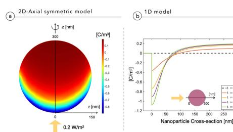
Fig. 2 Charge density distribution across the NP irradiated by a light intensity of 0.2 W m<sup>-2</sup> impinging as depicted by the yellow arrow. (a) Results obtained using the 2DAS NP model. (b) Results obtained using the 1D-model as a function of time after the illumination.
