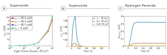
Fig. 5 (a) Superoxide concentration as a function of the proteinic concentration and the light intensity impinging onto the NP. (b) Profile of superoxide  $c_{0,-}(0^+,t)$  as a function of time at different light intensities. (c) Variation of hydrogen peroxide concentration  $\delta c_{\text{H}_2\text{O}_2}$  secondary to the production of superoxide.
