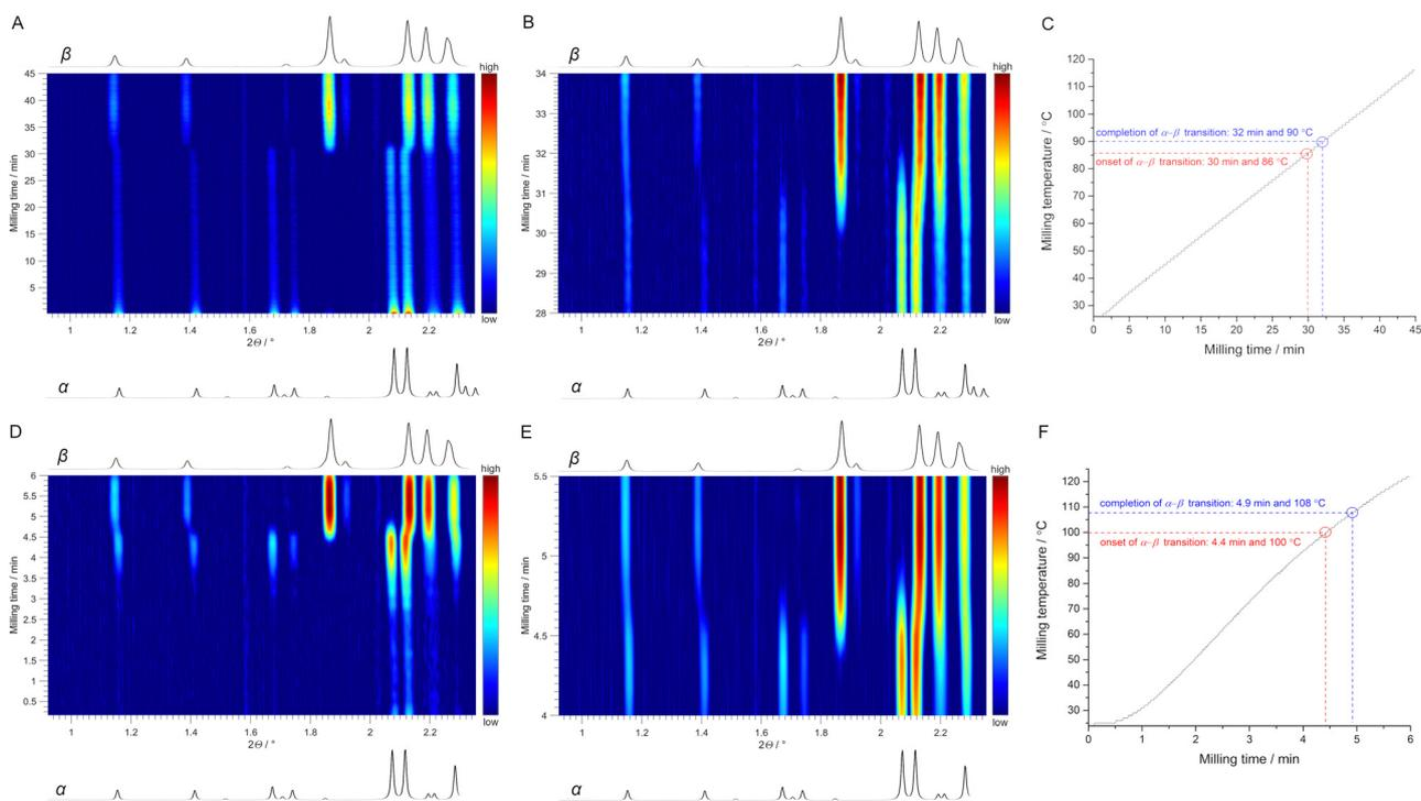
Fig. 4 *In situ* monitoring of milling ADE under different heating regimes by synchrotron PXRD ( $\lambda = 0.20741\text{ \AA}$ ). (A) With ramp heating. (B) Zoomed in region of (A). (C) Plotted data for milling temperatures associated with (A) and (B). (D) Heating without ramp. (E) Zoomed in region of (D). (F) Plotted data for milling temperatures associated with (D) and (E).
