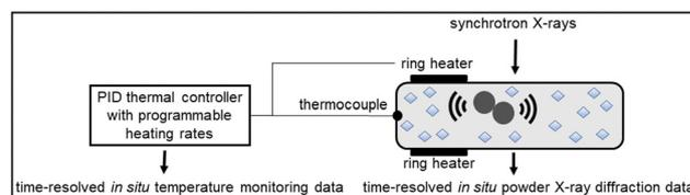
**Fig. 1** Our setup for direct measurement of polymorphic transition temperatures under thermo-mechanochemical conditions by simultaneous *in situ* synchrotron powder X-ray diffraction and temperature monitoring.
