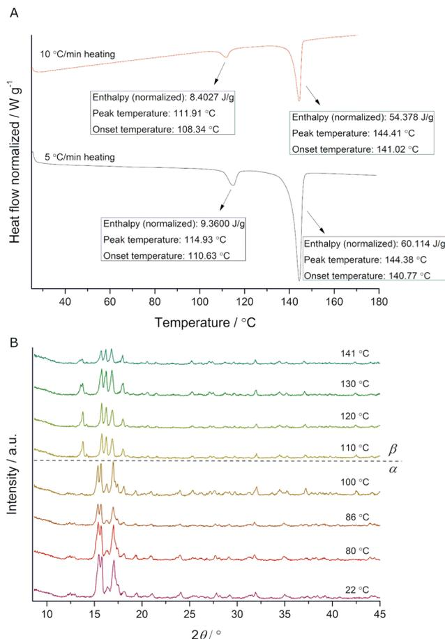
Fig. 2 (A) DSC traces of **ADE** obtained by applying different heating rates. Endotherms are pointing downwards. (B) *In situ* monitoring of **ADE** phase transition by VT-PXRD ( $\lambda = 1.54 \text{ \AA}$ ).
