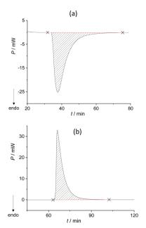
Fig. 1 (a) Thermogram for the formation of the metastable liquid BZP-DPA (n(BZP) = n(DPA) = 0.412 mmol) performed in the Setaram Calvet calorimeter at 25 °C. (b) Thermogram for the crystallization of the metastable liquid BZP-DPA (n(BZP) = n(DPA) = 0.314 mmol) forming BZP-DPA co-crystal performed in the Setaram Calvet calorimeter at 25 °C.
