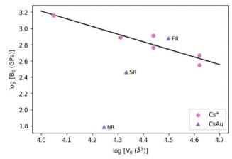
Fig. 2 Bulk modulus and unit cell volume of CsAu at the NR, SR, and FR approximations in comparison to alkali metal halides (top panel) and cesium halides (bottom panel).
