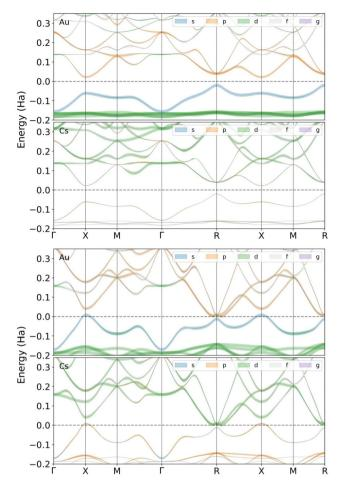
Fig. 5 Gold and cesium contributions to the electronic band structure of CsAu near the Fermi level at the SR approximation at zero pressure (top) and 31.5 GPa (threshold for metallization, bottom). Line thickness is proportional to each band's s, p, d, or f character. Energy is expressed relative to Fermi level.
