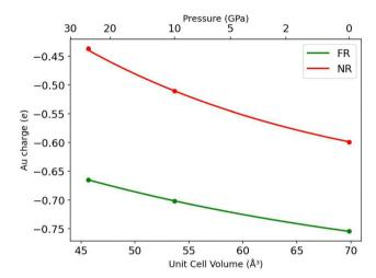
Fig. 7 Gold pseudo-charge from Bader analysis of CsAu in the  $Pm\overline{3}m$  structure at the NR and FR approximations. The pressure scale was calculated using the Vinet EOS fitted to FR data.
