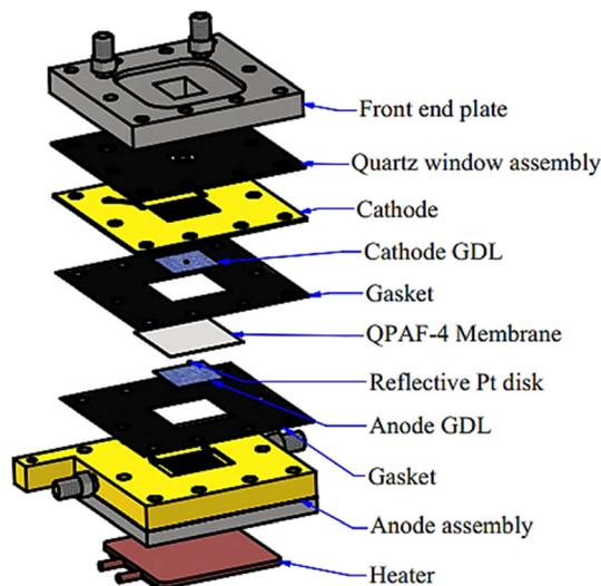
Fig. 2 Assembly of the fuel cell with a transparent quartz window, a hole in the GDL, and a reflective Pt disk.
