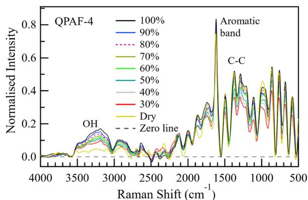
Fig. 13 Normalised Raman spectra from the centre of the QPAF-4 membrane at RH values 30–100% in steps of 10%. The spectra were normalised using the area under the aromatic band. A  $\times 50$  objective lens,  $100\text{ }\mu\text{m}$  hole, and D1 filter were used during the measurements.
