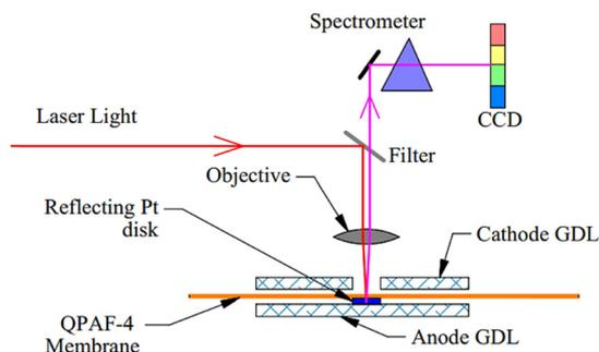
Fig. 3 Setup for micro-Raman spectroscopy. The red line shows the path of the 633 nm laser beam into the cell, and the pink line indicates the path followed by the generated signal into the spectrometer.
