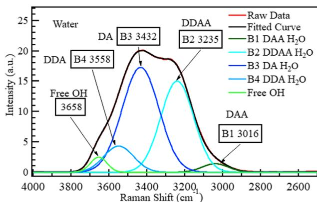
Fig. 6 The spectrum of liquid water deconvoluted into five Gaussian bands based on the Pezzotti assignments.<sup>48</sup> The raw data plot and fitted curve are also shown.
