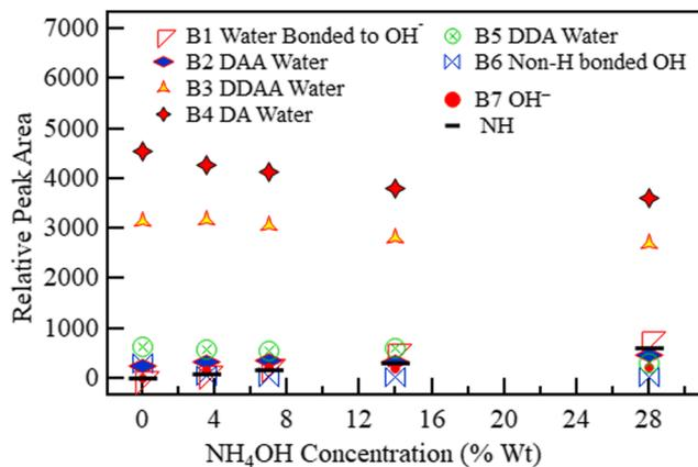
Fig. 12 The area under the six deconvoluted OH sub-bands within the OH band of aqueous  $\text{NH}_4\text{OH}$  with changing concentration. The 0 M concentration points refer to the spectrum of pure water.
