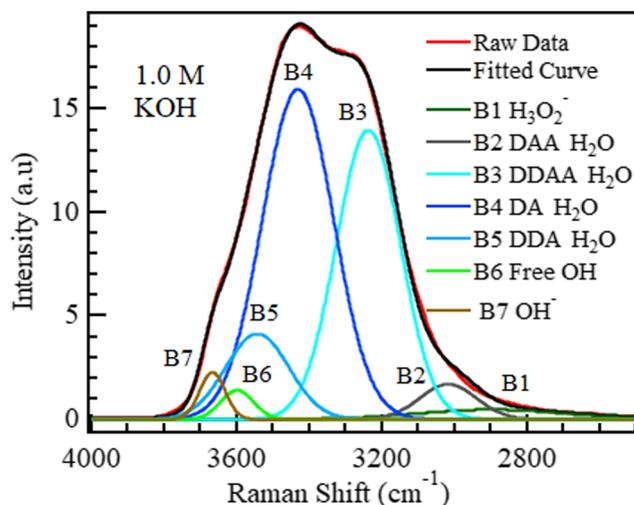
Fig. 7 1.0 M KOH spectrum deconvoluted into seven Gaussian bands.
