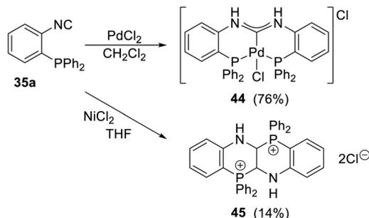
Scheme 13 Reactions of **35a** with PdCl<sub>2</sub> and NiCl<sub>2</sub>.
