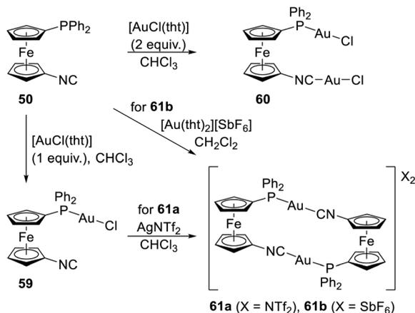
**Scheme 17** Preparation of Au(I) complexes featuring **50** as a ligand (NTf<sub>2</sub><sup>-</sup> = bis(trifluoromethanesulfonyl)imide anion, tht = tetrahydrothiophene).
