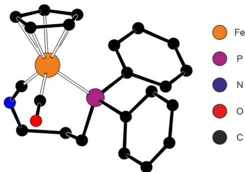
**Fig. 3** View of the complex cation in the structure of  $[(\eta^5\text{-C}_5\text{H}_5)\text{Fe}(\text{CO})(\text{Ph}_2\text{P}(\text{CH}_2)_3\text{NC-}\kappa^2\text{C,P})][\text{PF}_6]$  (**10a**). The diagram was drawn using the data deposited at the CCDC (deposition number: 1307387). One of two crystallographically independent cations is shown. Positions of the hydrogen atoms were not reported.
