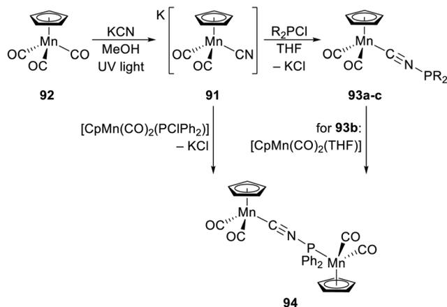
**Scheme 28** Synthesis and reactions of phosphinoisocyanide complexes **93a–c** [R = Et (a), Ph (b) and OEt (c)]. The preparation of **93a–c** was carried out at low temperature (–40 to –80 °C); the syntheses of **94** were performed in tetrahydrofuran (THF).
