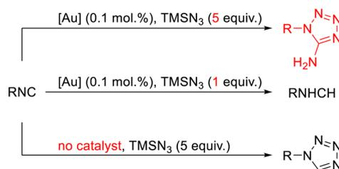
**Scheme 20** Divergent reactions of isocyanides with *in situ*-generated hydrazoic acid. All reactions were performed in dichloromethane/methanol. The noncatalysed reaction required considerably longer reaction times than the Au-mediated formation of aminotetrazoles did. [Au] = [Au(PPh<sub>3</sub>)(MeCN)][SbF<sub>6</sub>].
