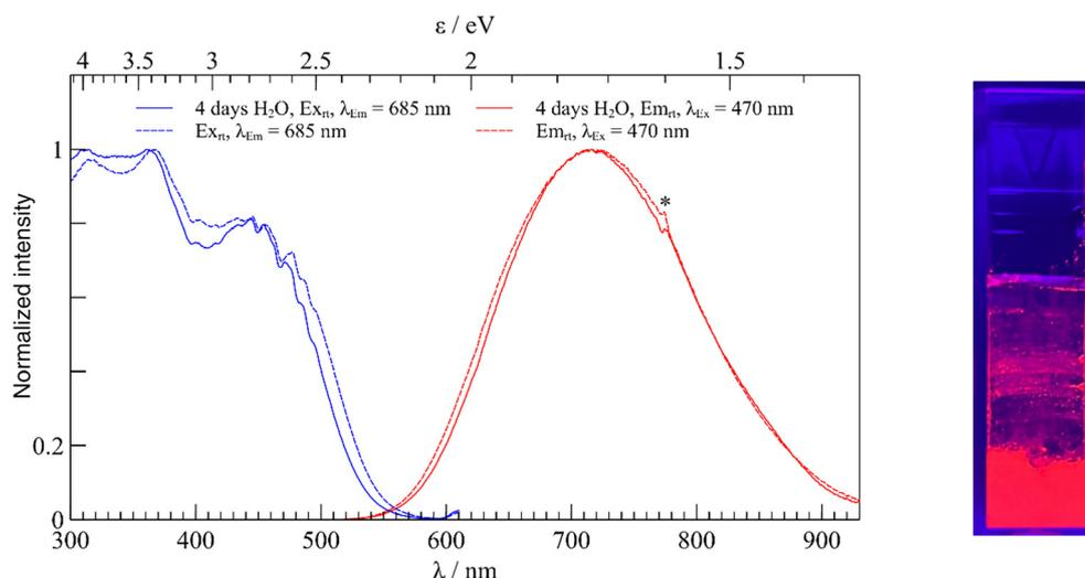
**Fig. 4** (Left) Normalized photoluminescence excitation (PLE (blue)) and emission (PL (red)) spectra of **1** in the solid state at room temperature before (dashed) and after 4 days immersed in H<sub>2</sub>O (solid). PLE was recorded with  $\lambda(\text{em}) = 685$  nm and PL with  $\lambda(\text{exc}) = 470$  nm. (Right) Cuvette with ground powder of **1** with added water.
