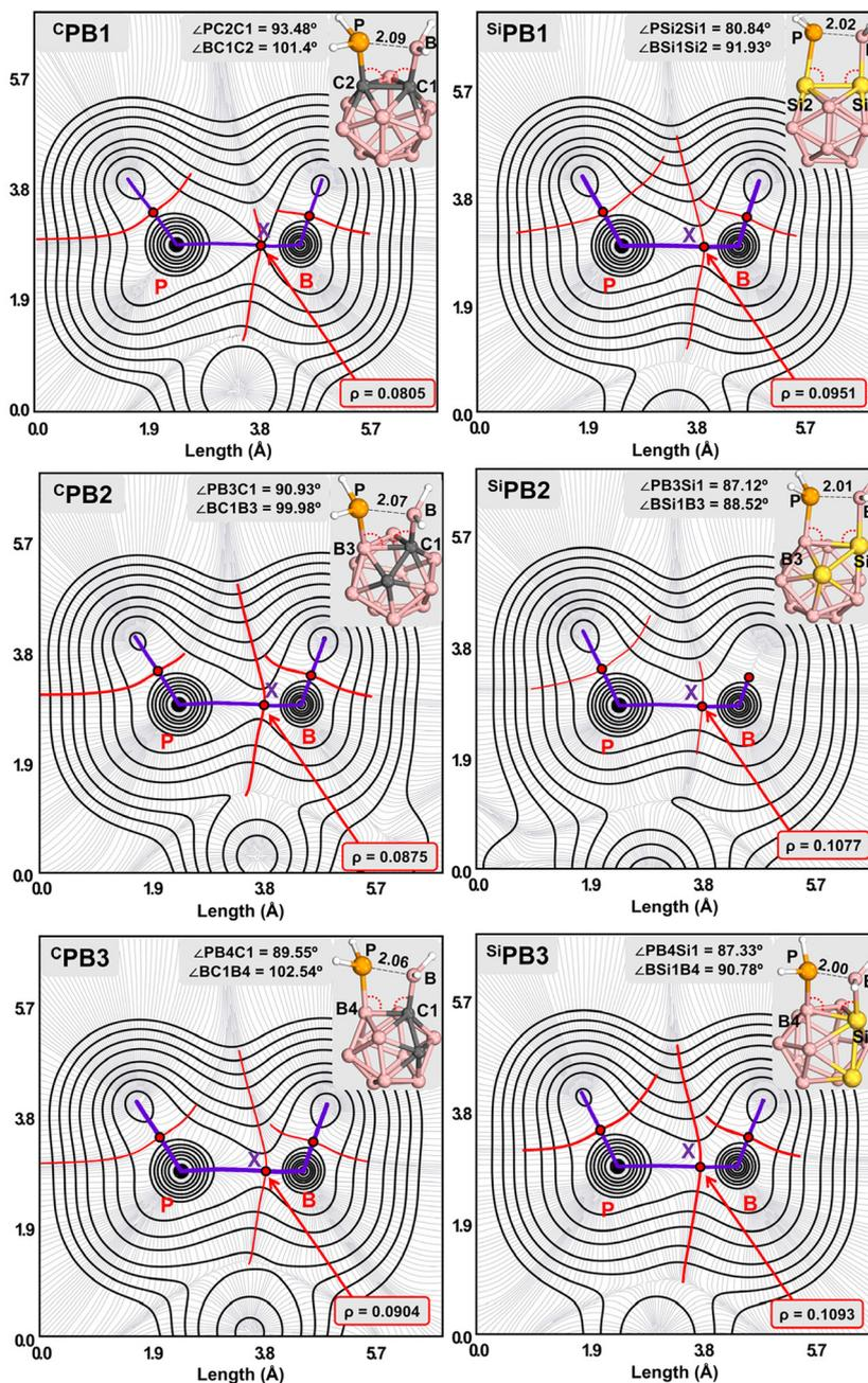
**Fig. 2** Electron density contour plots along with optimized geometries of <sup>Y</sup>PB<sub>n</sub> (Y = C, Si and n = 1–3) IFLPs. (The distances are in angstrom, red solid circles in the electron density plots represents bond critical point (BCP) X, electron density ( $\rho$ ) is in a.u., electron density was plotted at 0.001 a. u. iso value).
