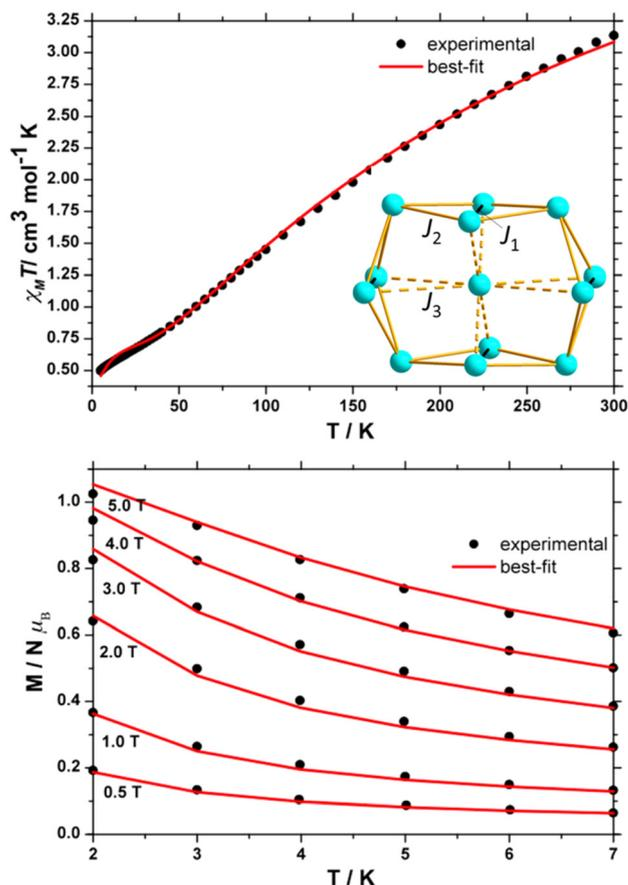
Fig. 9 Magnetic susceptibility (top) and magnetisation data (bottom) for **6**. The inset shows the exchange coupling scheme used to fit (solid red lines) the experimental data (black circles). Inset:  $J_1$  = solid black lines,  $J_2$  = solid gold lines,  $J_3$  = dashed gold lines. See text for details.
