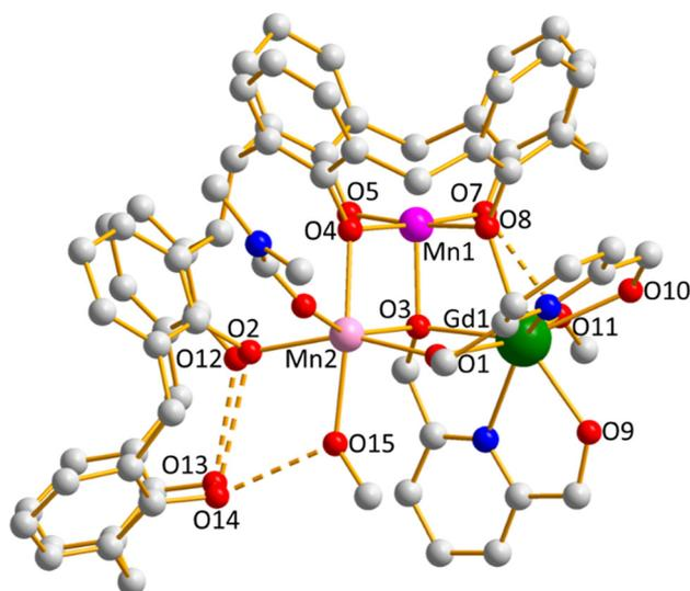
**Fig. 14** Molecular structure of complex **11**. Colour code: Gd<sup>III</sup> = dark green, Mn<sup>III</sup> = magenta, Mn<sup>II</sup> = pale pink, O = red, N = blue, Cl = light green, C = grey. H atoms, <sup>t</sup>Bu groups, endo-cavity solvent, and solvent of crystallisation are omitted for clarity.
