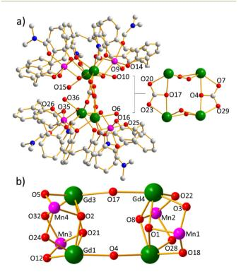
Fig. 12 (a) Molecular structure of complex 9. (b) The metal-oxygen core of 9. Colour code: Gd<sup>III</sup> = dark green, Mn<sup>III</sup> = magneta, O = red, N = blue, C = grey. H atoms, tBu groups and solvent of crystallisation omitted for clarity.
