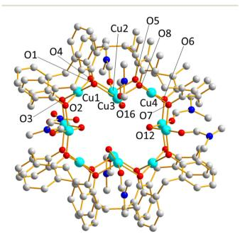
Molecular structure of complex 6. Colour code: Cu<sup>II</sup> = pale blue, O = red, N = dark blue, C = grey. The heavily disordered central Cu<sup>II</sup> atom, H atoms, tBu groups, counter ions, some endo-cavity solvent, and solvent of crystallisation are omitted for clarity.
