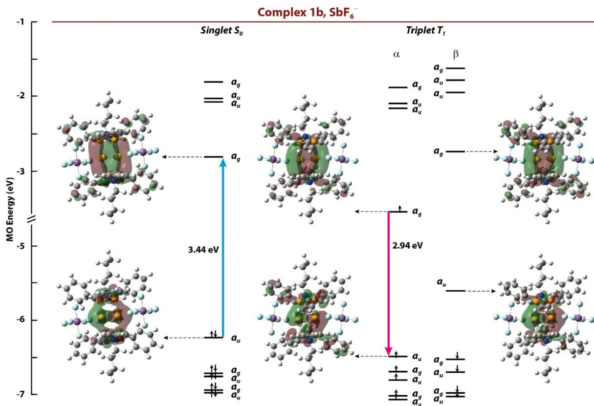
**Fig. 6** Frontier molecular orbitals (MOs) of **1b** calculated at the TPSSh level for the singlet ground state and the first triplet excited state ( $T_1$ ). The blue arrow indicates the  $S_0 \rightarrow S_1$  absorption transition and the red arrow describes the  $S_0 \leftarrow T_1$  emission transition.
