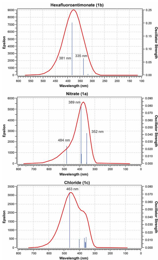
**Fig. 9** Theoretically predicted (TPSSh) UV/Vis absorption spectra of **1b**, **1a**, and **1c** (with  $R = n\text{Bu}$  and  $\text{SbF}_6^-$ ,  $\text{NO}_3^-$ , or  $\text{Cl}^-$  counterions, respectively).
