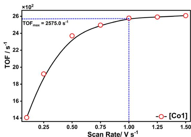
Fig. 8 Plot of TOF vs. scan rate for the calculation of TOF<sub>max</sub> for catalyst [Co1] under CO<sub>2</sub> saturated atmosphere in DMF medium.
