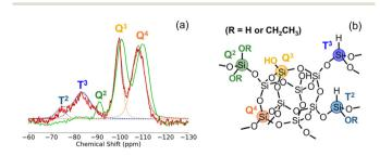
Fig. 2 (a) Solid-state <sup>29</sup>Si MAS NMR spectra of TES-Q8H8 (red) and Au/ TES-Q8H8 (green). Pale blue, blue, yellow and orange dotted lines respectively represent fitting data of TES-Q8H8 attributable to T2, T3, Q<sup>3</sup>, and Q<sup>4</sup> environments. (b) Si environment in the assumed structure
