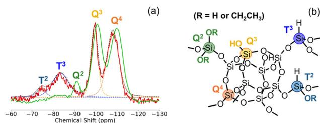
**Fig. 2** (a) Solid-state  $^{29}\text{Si}$  MAS NMR spectra of TES-Q8H8 (red) and Au/TES-Q8H8 (green). Pale blue, blue, yellow and orange dotted lines respectively represent fitting data of TES-Q8H8 attributable to  $\text{T}^2$ ,  $\text{T}^3$ ,  $\text{Q}^3$ , and  $\text{Q}^4$  environments. (b) Si environment in the assumed structure of TES-Q8H8.
