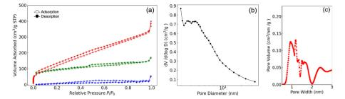
Fig. 3 (a) N<sub>2</sub> adsorption-desorption isotherms of TES-Q8H8 (red), Q8H8-only (blue), and TES-Q8H8-calc. (green). (b) Pore size distribution, as determined from BJH analysis of Adsorption data for TES-Q8H8. (c) Micro pore size distribution determined from SF analysis of TES-Q8H8.
