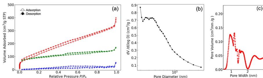
**Fig. 3** (a)  $N_2$  adsorption–desorption isotherms of TES-Q8H8 (red), Q8H8-only (blue), and TES-Q8H8-calc. (green). (b) Pore size distribution, as determined from BJH analysis of Adsorption data for TES-Q8H8. (c) Micro pore size distribution determined from SF analysis of TES-Q8H8.
